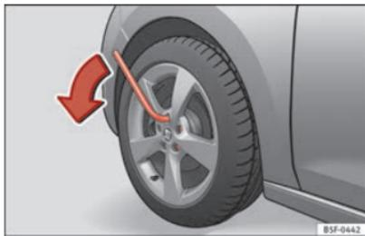
Fig. 173 Changing a wheel: loosen the wheel bolts.
