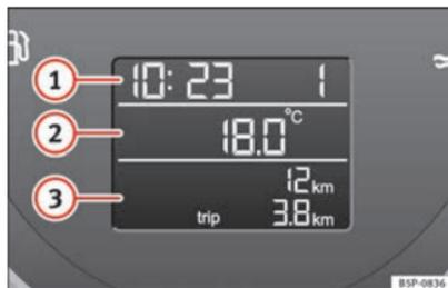
Fig. 38 Detailed view of the instrument panel: screen with different indicators.
