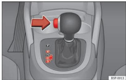
Fig. 142 Centre console: Automatic gearbox selector lever
