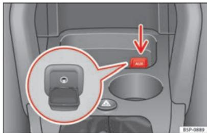
**Fig. 113 Auxiliary audio connection**
