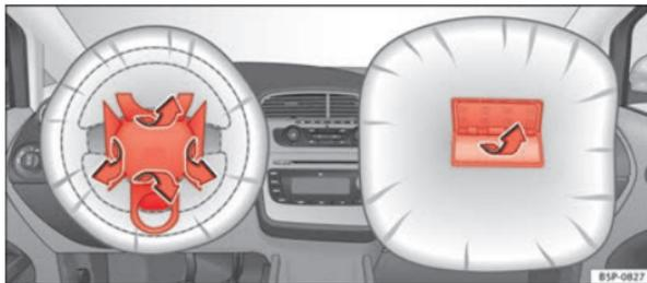
Fig. 21 Airbag covers during deployment of front airbags.
