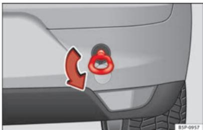
**Fig. 211** Fitting the towline anchorage to the rear of the vehicle.
