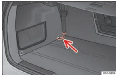
Fig. 122 Fastening rings to tighten partition net.
