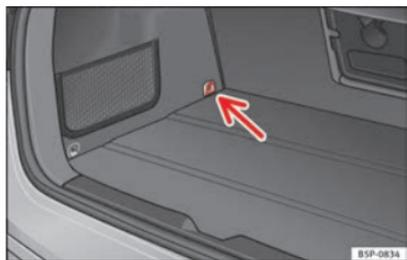
Fig. 32 Top Tether\* securing ring.
