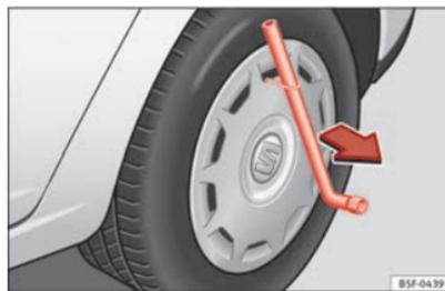
Fig. 172 Changing a wheel: remove the wheel cover.
