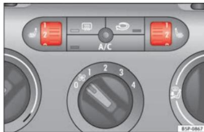
Fig. 88 Thumb wheel for the front seat heating
