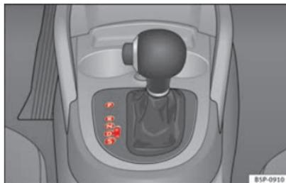
Fig. 140 Centre console: Selector lever for automatic gearbox / DSG automatic gearbox
