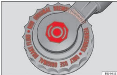
Fig. 167 Engine compartment: brake fluid reservoir lid.
