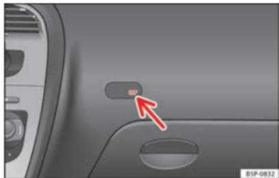
Fig. 23 Control lamp for deactivated front passenger airbag.
