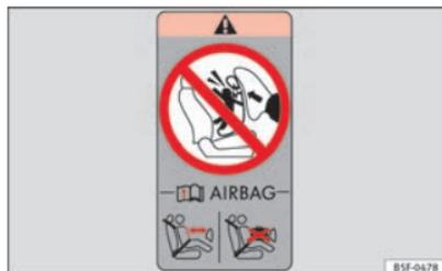
Fig. 17 On the rear frame of the passenger side door: airbag sticker.
