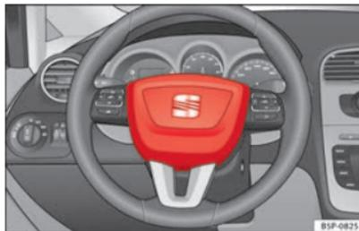
Fig. 18 Driver airbag located in steering wheel.
