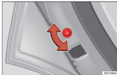
**Fig. 57 Childproof lock on the left hand side door.**
