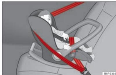
Fig. 28 A group 0 rear-facing child seat fitted on the rear seat ▶
