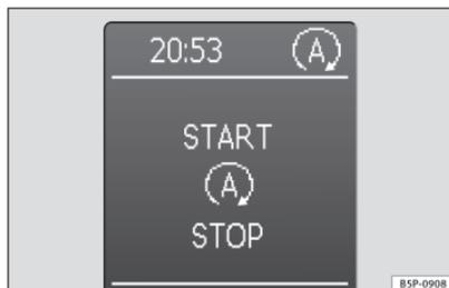
Fig. 138 Display on the instrument panel during Start-Stop function operation.
