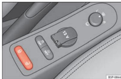
Fig. 55 Detailed view of the centre console: central locking button.
