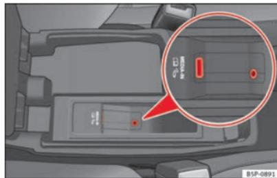
**Fig. 115 Connection in central armrest compartment**
