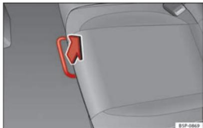
Fig. 90 Rear seat unlocking bar
