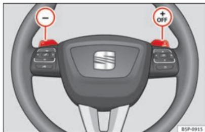
Fig. 144 Steering wheel with levers for automatic gearbox.
