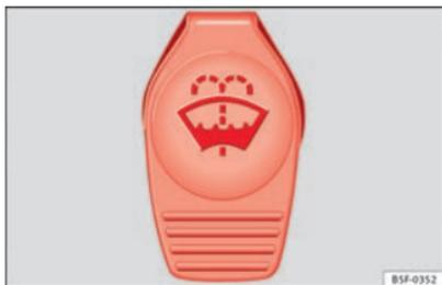
Fig. 162 In the engine compartment: Cap of windscreen washer fluid reservoir
