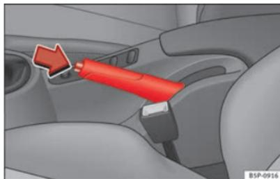
Fig. 145 Handbrake between the front seats.
