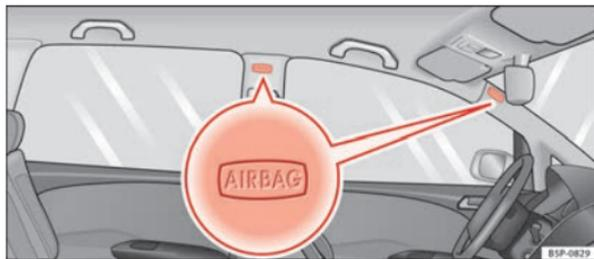
Fig. 26 Location of curtain airbags on the left side of the vehicle
