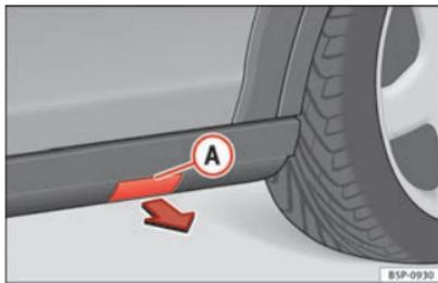
Fig. 176 Plastic sill panel trim with jack allotment cover
