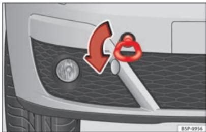
**Fig. 210** The front right section of the vehicle: Fitting the front towline anchorage
