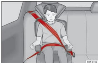
Fig. 30 Forward-facing child seat installed on rear seat
