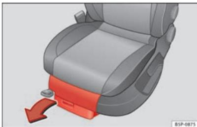
Fig. 96 Storage compartment under the front seats
