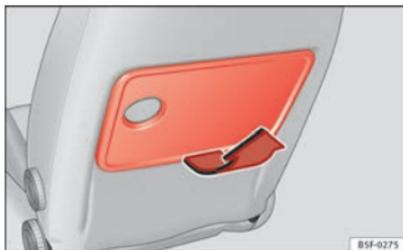
Fig. 97 Folding tray on the front left seat
