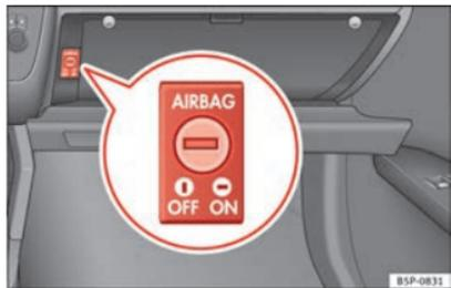
Fig. 22 In the glove compartment: key-operated switch for activating and deactivating the front passenger airbag.
