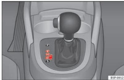
Fig. 141 Centre console: Automatic gearbox selector lever
