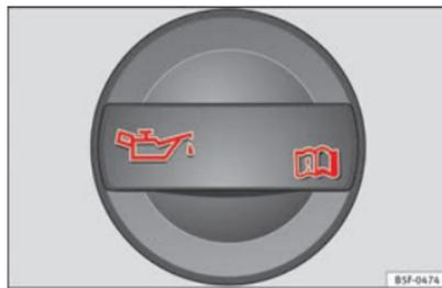
Fig. 160 Engine oil filler cap in the engine compartment.
