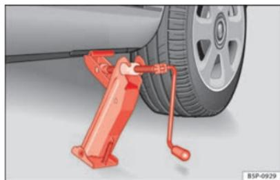
Fig. 175 Fitting the jack.
