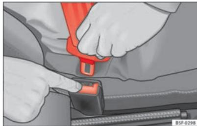
Fig. 12 Remove latch plate from the buckle.
