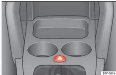
Fig. 72 Dash panel: switch for hazard warning lights.
