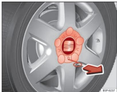
Fig. 171 Changing a wheel: removing a hub cap
