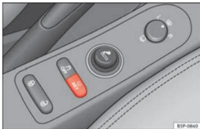
Fig. 48 Centre console: tyre monitor system button.
