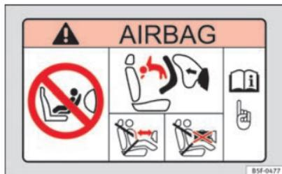
Fig. 16 Passenger side sun visor: airbag sticker.
