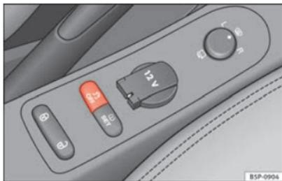
**Fig. 134 Detailed view of the centre console: ESC switch.**
