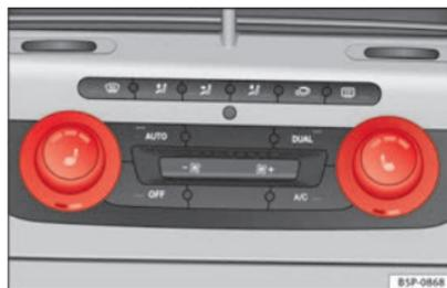
Fig. 89 Climatronic front seat heating
