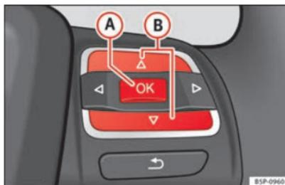
Fig. 45 Controls on the steering wheel: control buttons.
