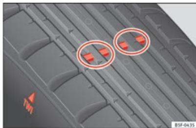
Fig. 168 Tyre tread wear indicators.
