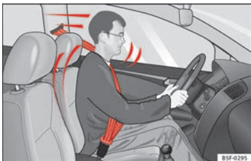
Fig. 87 Drivers with properly worn seat belts will not be thrown forward in the event of sudden braking
