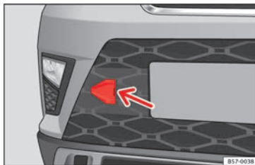
Fig. 96 Front bumper on right: remove the lid.
