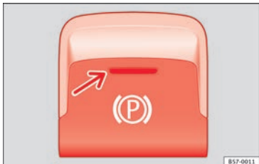
Fig. 165 In the lower part of the centre console: electronic parking brake button.
