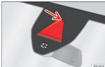
Fig. 191 In the windscreen: field of vision of the Lane Assist system camera.
