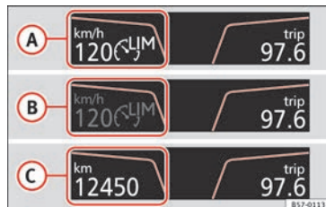
Fig. 172 On the instrument panel display: messages on the status of the speed limiter.
