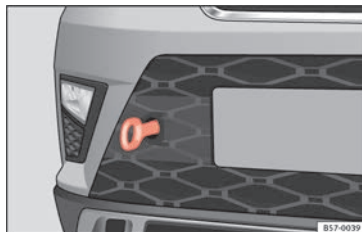
Fig. 74 Right side of the front bumper: towline anchorage screwed in.
