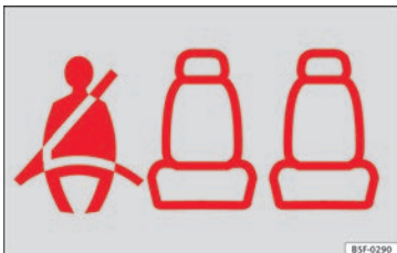
Fig. 86 Instrument panel: right rear seat occupied and corresponding seat belt fastened display.
