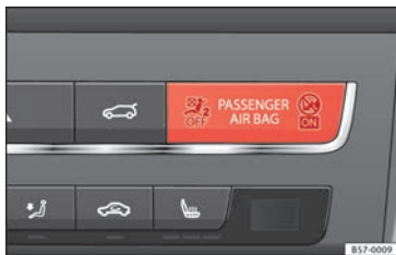
Fig. 92 Control lamp for disabling the front passenger front airbag on the dash panel
