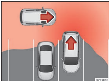
Fig. 196 Schematic representation of the rear cross traffic alert: monitored zone around the vehicle being parked.
