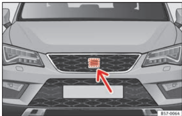
Fig. 177 On the front behind the SEAT badge: radar sensor.
