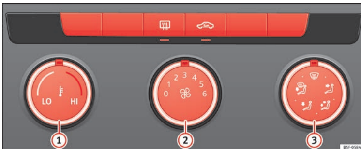
Fig. 57 In the centre console: heating system and fresh air controls.
