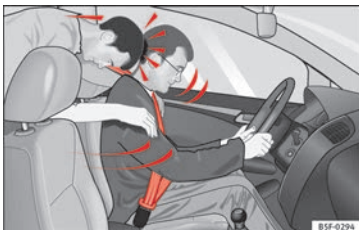
Fig. 89 The unbelted passenger in the rear seat is thrown forward violently, hitting the driver who is wearing a seat belt.
