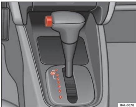
Fig. 99 Centre console: Automatic gearbox selector lever
