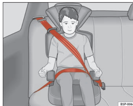
Fig. 29 Forward-facing child seat installed on rear seat.
