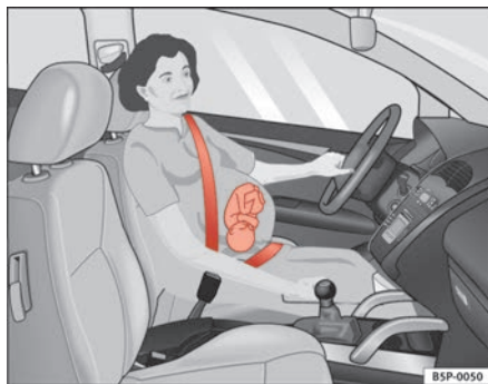
Fig. 14 Positioning seat belts during pregnancy
