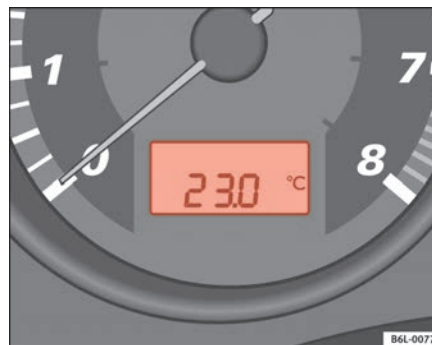
Fig. 38 Digital instrument panel display: outside temperature display.
