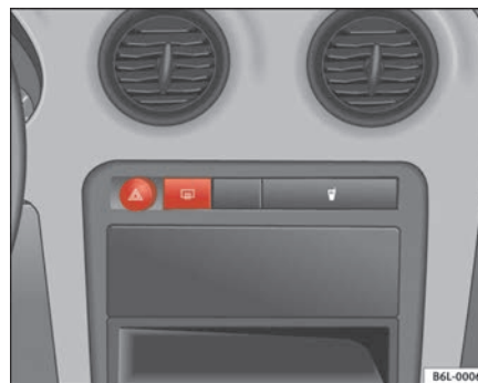
Fig. 58 Instrument panel: heated rear window switch
