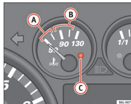
Fig. 33 Engine coolant temperature
