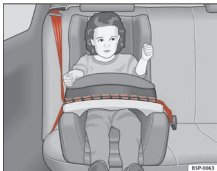
Fig. 28 A category 1 forward-facing child seat fitted on the rear seat.
