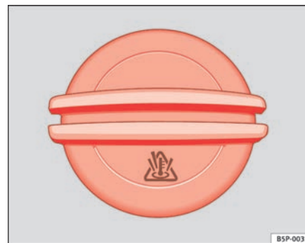
Fig. 125 In the engine compartment: Coolant expansion tank cap
