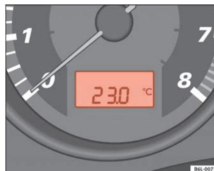
Fig. 36 Digital instrument panel display: Outside temperature display
