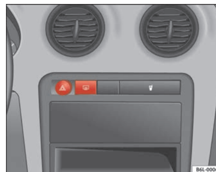
Fig. 59 Instrument panel: switch for hazard warning lights
