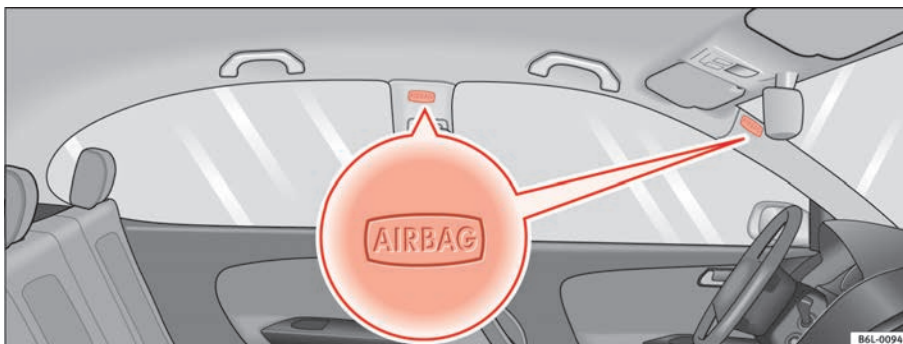
Fig. 23 Location of left curtain airbag
