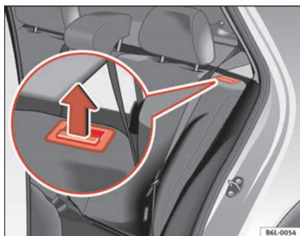
Fig. 75 Button for unlocking the rear backrest
