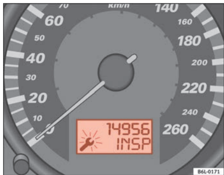
Fig. 39 Service interval display
