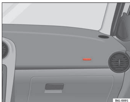
Fig. 18 Front passenger airbag located in dash panel
