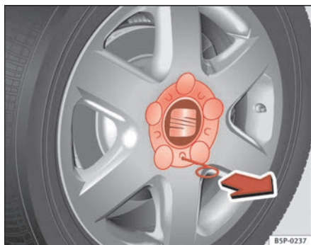
Fig. 131 Changing the wheel: Removing a hub cap
