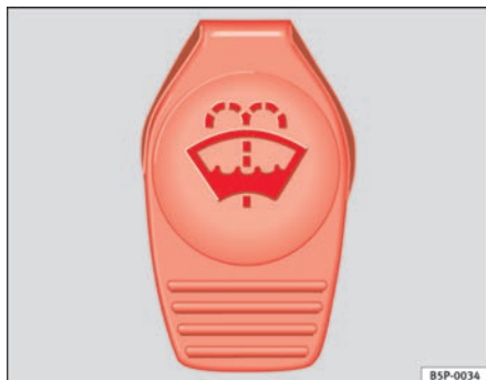
Fig. 126 In the engine compartment: Cap of windscreen washer fluid reservoir.
