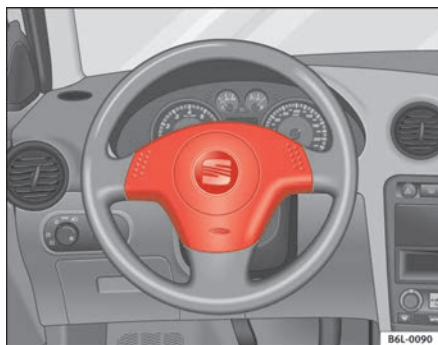
Fig. 17 Driver airbag located in steering wheel
