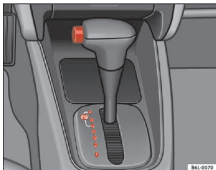
Fig. 98 Centre console: Automatic gearbox selector lever
