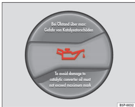
Fig. 124 In the engine compartment: Engine oil filler cap
