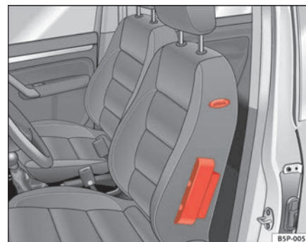
Fig. 21 Side airbag in driver seat
