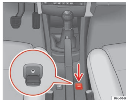
Fig. 84 Auxiliary audio connection
