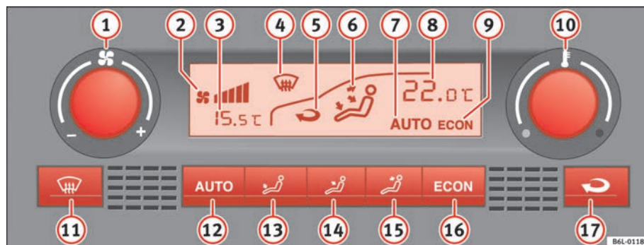
Fig. 92 On the instrument panel: Climatronic controls
