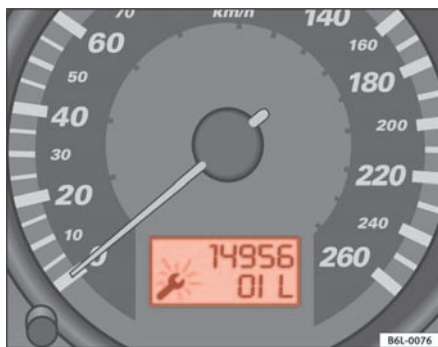
Fig. 39 Service interval display
