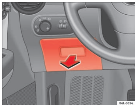
Fig. 77 Driver's side compartment
