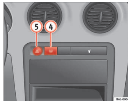
Fig. 58 Instrument panel: rear window heater switch
