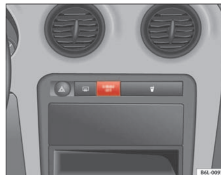
Fig. 26 Warning lamp for deactivated passenger airbag in centre console
