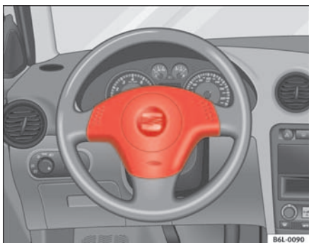
Fig. 17 Driver airbag located in steering wheel
