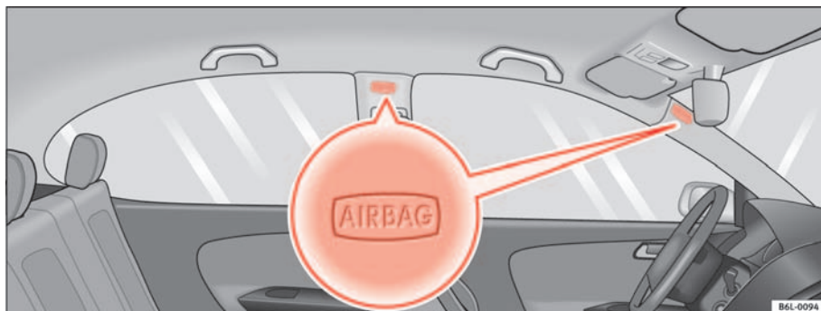
Fig. 23 Location of left curtain airbag
