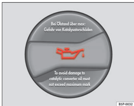
Fig. 123 In the engine compartment: Engine oil filler cap
