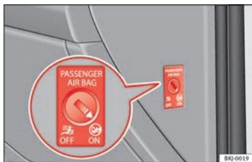
Fig. 105 Switch for activating and deactivating the front passenger airbag.
