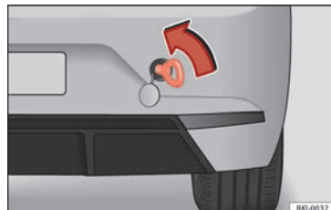
Fig. 88 Right side of the rear bumper: Towing ring.
