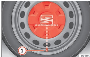
Fig. 78 Correct positioning of the central wheel trim for steel rims.
