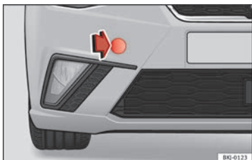
Fig. 108 Right side of the front bumper: remove the lid.
