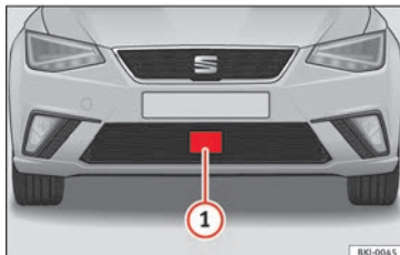
Fig. 192 On the front bumper: radar sensor.
