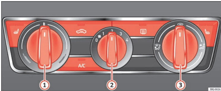
Fig. 63 In the centre console: Manual air conditioning controls.
