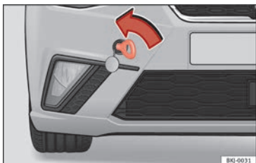
Fig. 109 Right side of the front bumper: towline anchorage screwed in.
