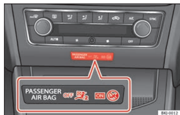
Fig. 57 Warning lamp for disabling the front passenger airbag.
