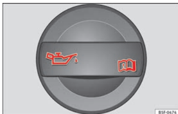
Fig. 67 In the engine compartment: Engine oil filler cap.
