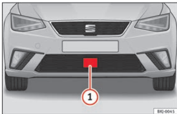
Fig. 197 On the front bumper: radar sensor.
