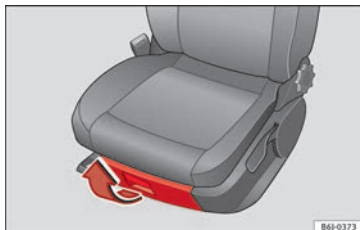
Fig. 160 Storage compartment under the right front passenger seat.
