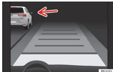
Fig. 200 On the instrument panel display: ACC active, vehicle detected in an outer lane.
