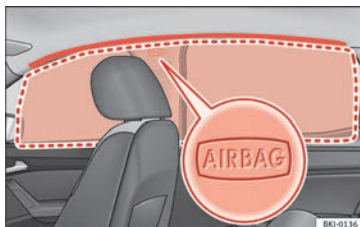
Fig. 27 Location and deployment area of the head-protection airbag.
