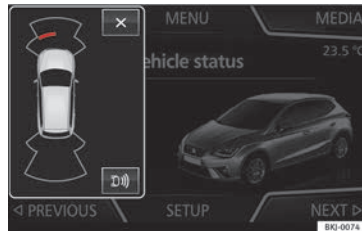
Fig. 208 Miniature indication of automatic activation.
