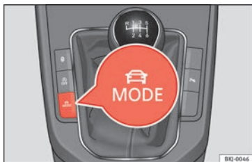
Fig. 203 Next to the gearbox lever: MODE button.
