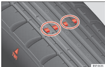
Fig. 232 Tyre tread wear indicators.
