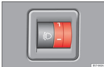
Fig. 150 Dash panel: headlight range control.
