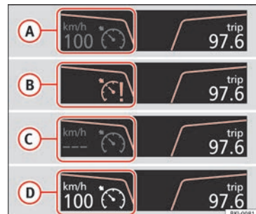
Fig. 187 Instrument panel display: CCS status indications.
