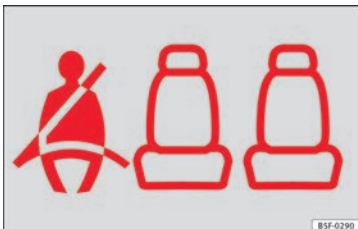
Fig. 99 Instrument panel: right rear seat occupied and corresponding seat belt fastened display.
