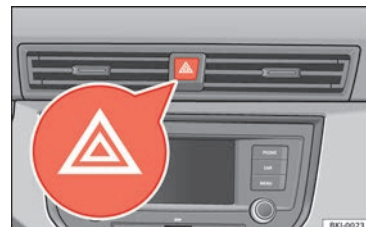
Fig. 42 Dash panel: switch for hazard warning lights.
