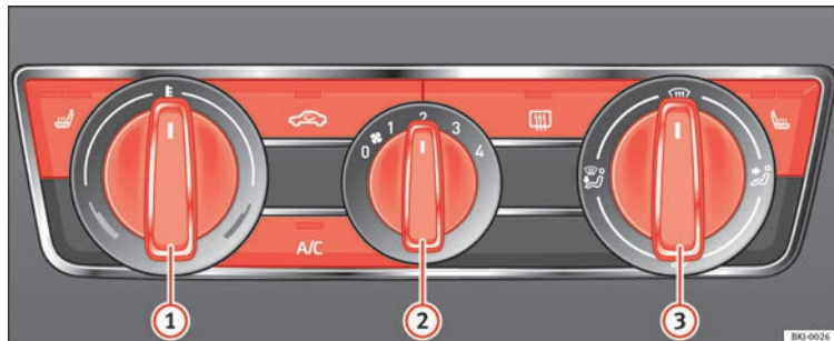
Fig. 175 Air conditioning controls on the dash panel.
