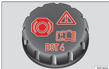
Fig. 69 Engine compartment: brake fluid reservoir cap.
