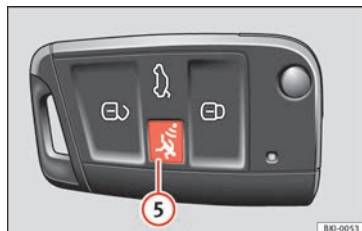
Fig. 137 Vehicle key with alarm button.
