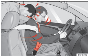
Fig. 102 The unbelted passenger in the rear seat is thrown forward violently, hitting the driver who is wearing a seat belt.
