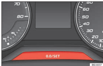
Fig. 126 Instrument panel: odometer and reset button.
