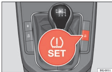
Fig. 234 Centre console: tyre monitoring system button.
