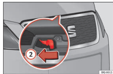
Fig. 10 Lever under the bonnet.
