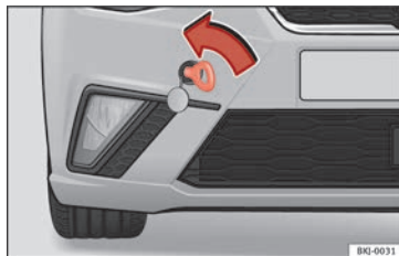
Fig. 87 Right side of the front bumper: Towing ring.
