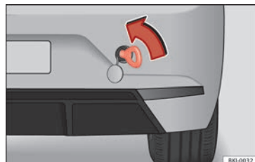
Fig. 111 Right side of the rear bumper: towline anchorage screwed in.
