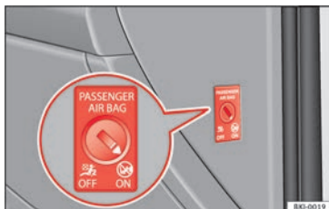
Fig. 23 Front passenger front airbag switch.
