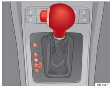
Fig. 116 Changing gear with tiptronic
