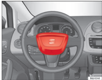
Fig. 16 Driver airbag located in steering wheel
