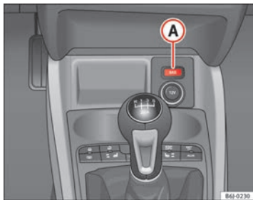
Fig. 108 Centre console: gas system control switch.
