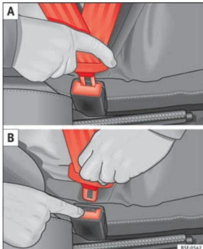
**Fig. 91** Positioning and removing the seat belt buckle.
