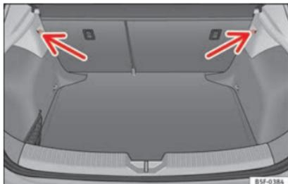
**Fig. 176** In the luggage compartment: retaining hooks (LEON/LEON SC model).
