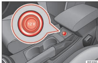
**Fig. 158** Centre console: front/rear 12-volt power socket.
