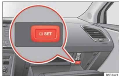
**Fig. 254** Glove compartment: tyre control switch.
