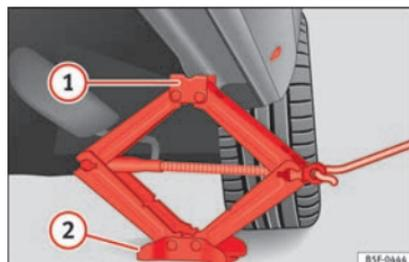
**Fig. 74** Strut: mounting the jack on the vehicle.
