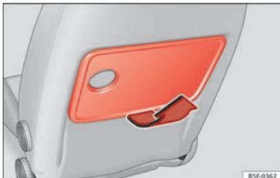
Fig. 155 Left-hand front seat: folding table.
