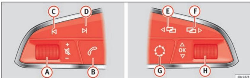
Fig. 124 Controls on the steering wheel.
