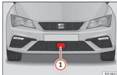
**Fig. 212** On the front bumper: radar sensor.
