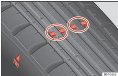
**Fig. 251** Tyre tread: tread wear indicators
