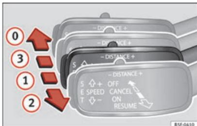
**Fig. 204** On the left of the steering column: third lever for operating the Adaptive Cruise Control.
