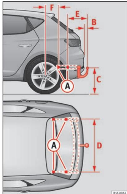
Fig. 245 Attachment points for towing bracket.
