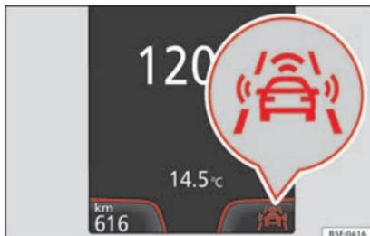
**Fig. 213** On the instrument panel display: Front Assist switched off message.
