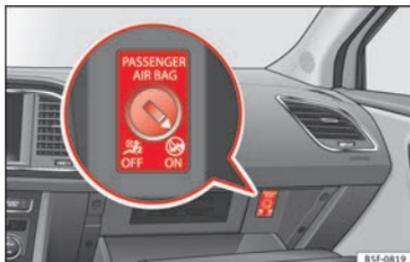
Fig. 22 Front passenger front airbag switch.
