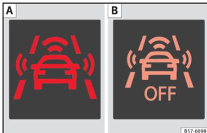
**Fig. 215** On the instrument panel display: **A** Advance warning message. **B** Pedestrian Monitoring deactivated.
