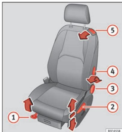
Fig. 13 Front seats: manual seat adjustment.
