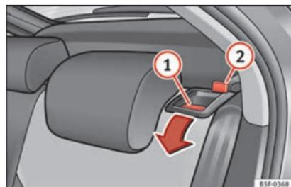
Fig. 151 Backrest release lever.
