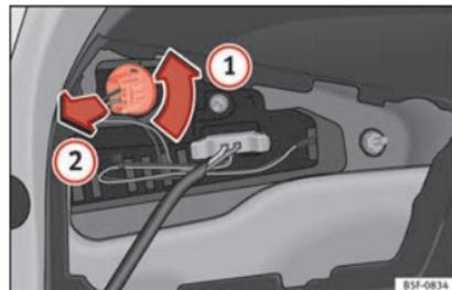
**Fig. 116** Remove the bulb holder.
