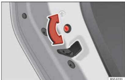
**Fig. 136** Childproof lock on the left hand side door.
