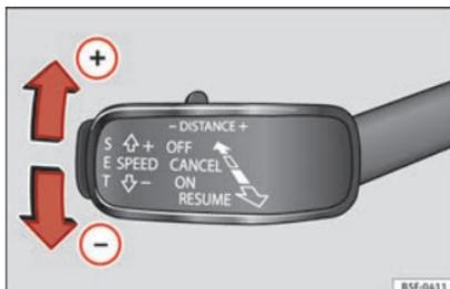
**Fig. 205** On the left of the steering column: third lever for operating the Adaptive Cruise Control.
