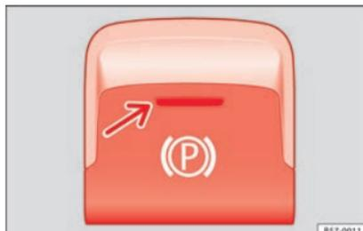
**Fig. 191** In the lower part of the centre console: electronic parking brake button.
