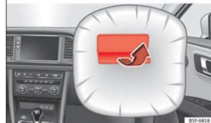
**Fig. 21** Front passenger airbag located in dash panel.
