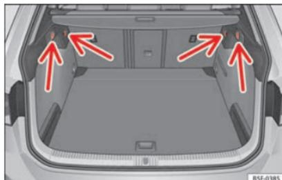
**Fig. 177** In the luggage compartment: retaining hooks (LEON ST model).
