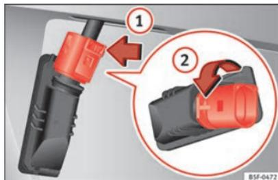
**Fig. 118** Number plate light: Remove the bulb holder.
