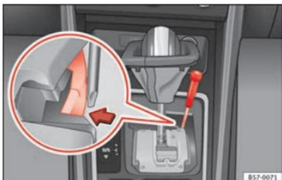
**Fig. 54** Selector lever: manual release from position P.
