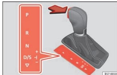
**Fig. 53** Automatic gearbox: selector lever positions.
