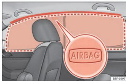
Fig. 27 Location of head-protection airbags.
