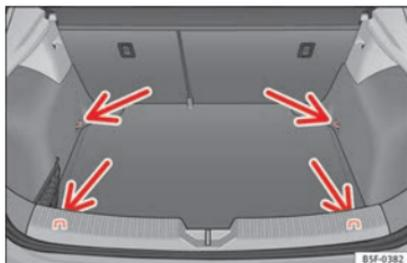
Fig. 174 In the luggage compartment: fastening rings (LEON/LEON SC model except versions with spare wheel and CNG).
