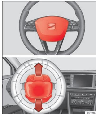
**Fig. 20** Driver airbag located in steering wheel.
