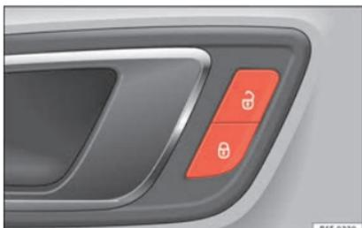
Fig. 2 Driver door: central locking switch.
