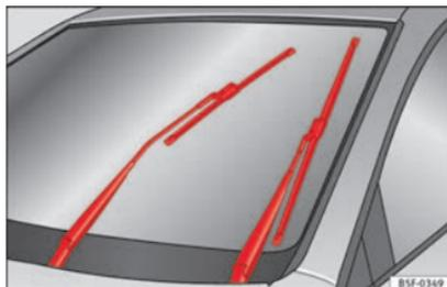
Fig. 79 Wipers in service position.
