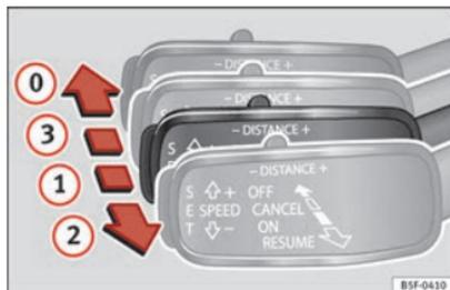
**Fig. 206** On the left of the steering column: third lever for operating the Adaptive Cruise Control.
