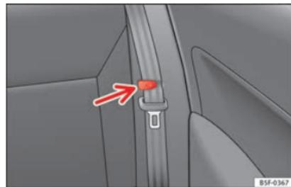
Fig. 150 Clip to support the seat belt.
