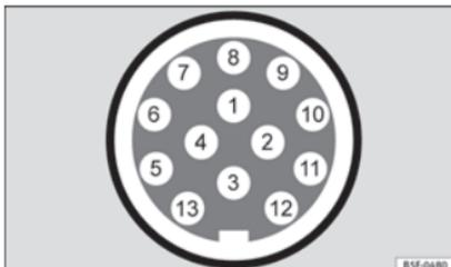
**Fig. 243** Schematic diagram: assignment of the pins of the trailer's electrical socket.
