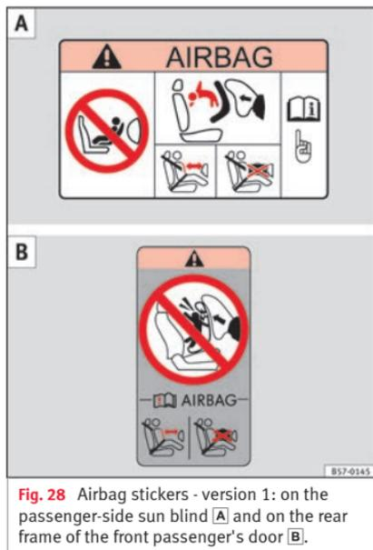
**Fig. 28** Airbag stickers - version 1: on the passenger-side sun blind [A] and on the rear frame of the front passenger's door [B].
