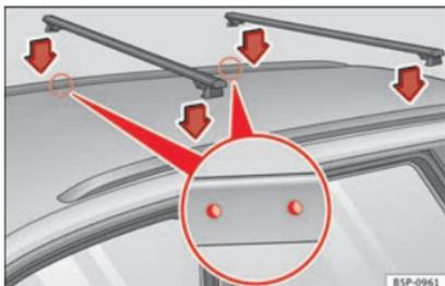
**Fig. 185** Leon ST: attachment points for the roof railings for the roof carrier system.
