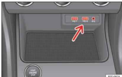
**Fig. 126** Centre console: USB/AUX-IN input.
