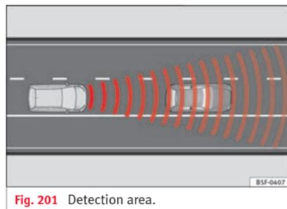
The adaptive cruise control (ACC) **is an extension of the normal cruise control system (CCS)** » ⚠.
