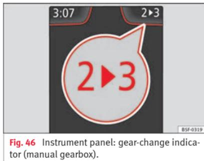
**Fig. 46** Instrument panel: gear-change indicator (manual gearbox).
