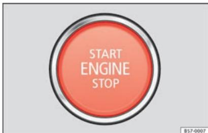
**Fig. 188** In the lower part of the centre console: starter button.
