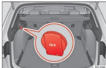
**Fig. 159** Detailed view of the side trim in the luggage compartment: 12-volt power socket (applies only to the LEON ST model).
