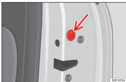
**Fig. 4** Locking the door manually.
