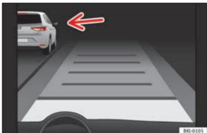
**Fig. 208** On the instrument panel display: ACC active, vehicle detected in an outer lane.
