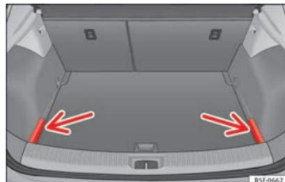
**Fig. 164** In the luggage compartment: covers for storing the rear shelf.
