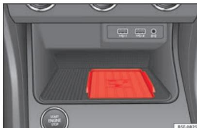
**Fig. 128** Centre console: Connectivity Box.
