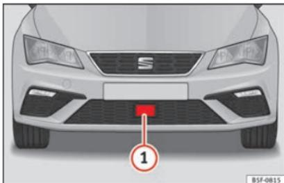
Fig. 203 On the front bumper: radar sensor.
