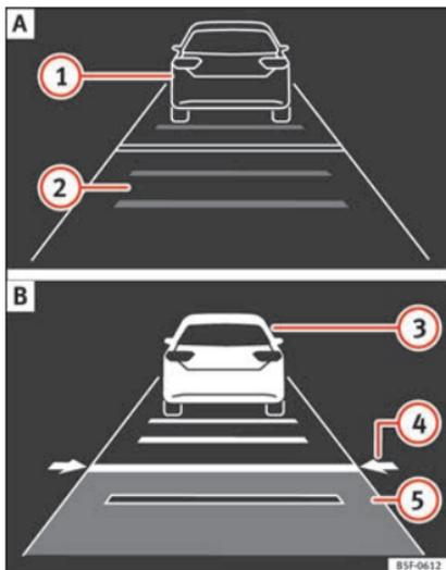
**Fig. 202** On the instrument panel display: (A) ACC temporarily inactive, vehicle detected in front, temporary distance adjusted. (B) ACC active, vehicle detected in front, temporary distance adjusted.
