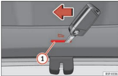
**Fig. 6** Luggage compartment: access to manual release.
