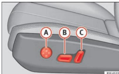
Fig. 14 Driver's seat: electric seat adjustment.
