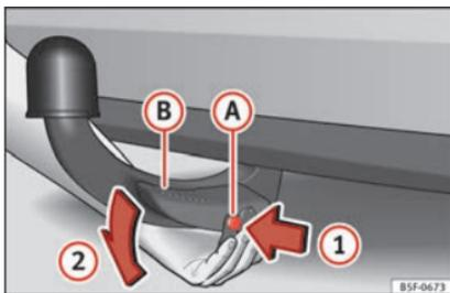
Fig. 242 Releasing the detachable ball.
