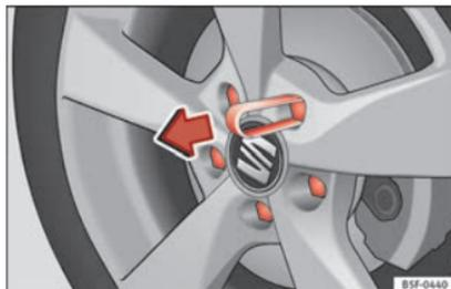
**Fig. 70** Wheel: wheel bolts with caps.
