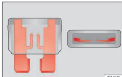
**Fig. 66** Image of a blown fuse.
