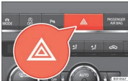
**Fig. 140** Dash panel: switch for hazard warning lights.
