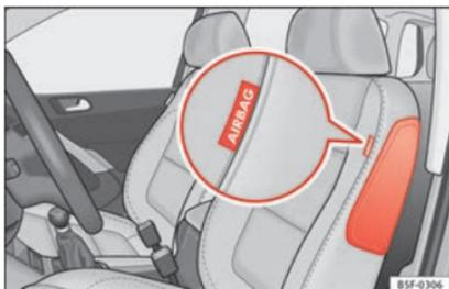
Fig. 25 Side airbag in driver's seat.
