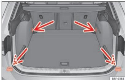
Fig. 175 In the luggage compartment: fastening rings (LEON ST model).
