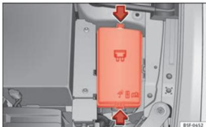
**Fig. 65** In the engine compartment: fuse box cover.
