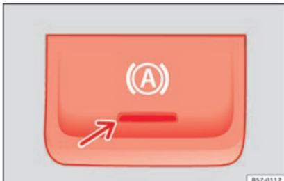
**Fig. 198** In the lower part of the centre console: Auto Hold function button.
