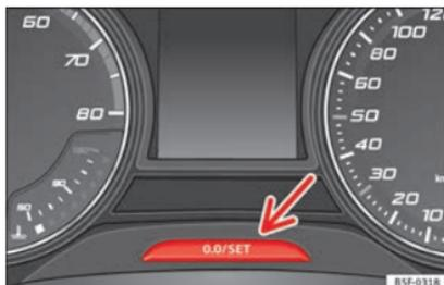
**Fig. 121** Instrument panel: odometer and reset button.
