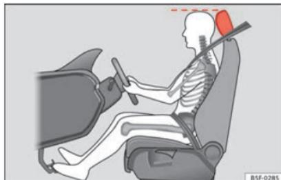
**Fig. 83** Correct head restraint position for the driver.
