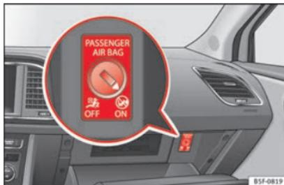
**Fig. 94** Front passenger front airbag switch.
