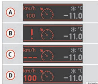
Fig. 199 Instrument panel display: CCS status indications.
