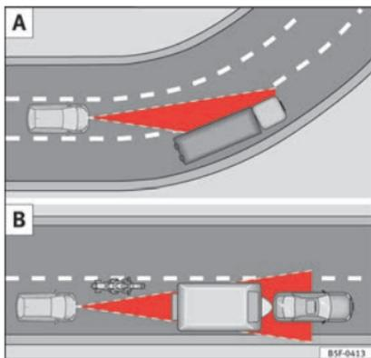
**Fig. 209** (A) Vehicle on a bend. (B) Motorcyclist ahead out of range of the radar sensor.
