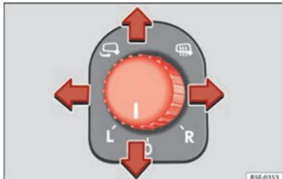
**Fig. 146** Driver door: control for the exterior mirror.
