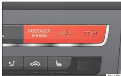
**Fig. 95** Warning lamp for disabling the front passenger airbag.
