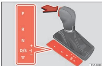
Fig. 194 Selector lever lock.
