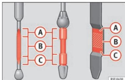
Fig. 59 Engine oil dipstick.
