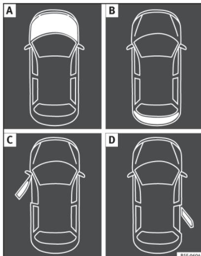
**Fig. 45** A: bonnet open; B: rear lid open; C: front left door open; D: rear right door open (5-door vehicles only).
