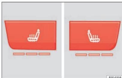
Fig. 148 In the centre console: front seats heating switch
