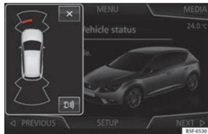
**Fig. 227** Miniature indication of automatic activation.
