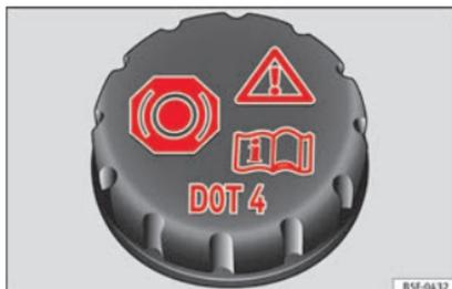
**Fig. 62** Engine compartment: brake fluid reservoir cap.
