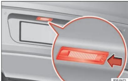
**Fig. 117** In the rear bumper: number plate light.
