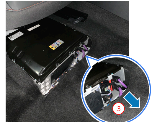
Disconnecting the 48-volt vehicle electrical system in mild hybrid vehicles (MHEV).
