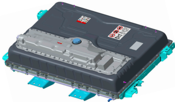
Example of a high-voltage battery for the LEON eHybrid
