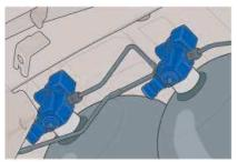
Electromagnetic shut-off valves on the gas tanks
