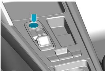
Press START-STOP button without operating the brake pedal
