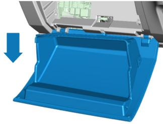
To return the glove box to the service position, release the side retaining tabs.
