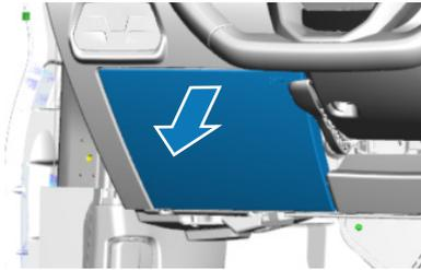
Release the cover next to the steering column with a screwdriver
