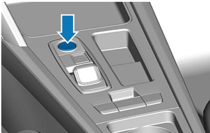
Press the START - ENGINE - STOP button located in the center console without pressing the brake pedal.
