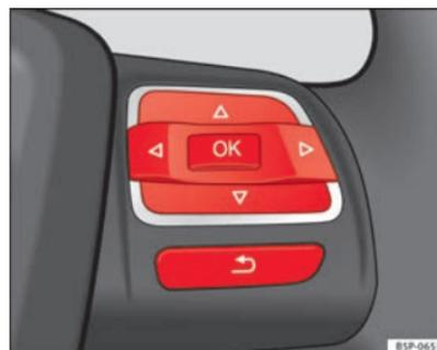
Fig. 3 Right-side buttons on the multifunction steering wheel.
