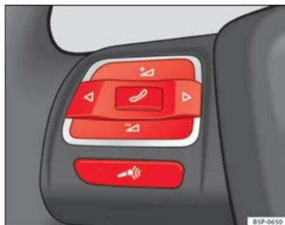
Fig. 2 Left-side buttons on the multifunction steering wheel.
