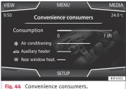
By pressing the <u>(Consumers</u>) button, information on the status of the vehicle's main consumption devices is obtained. It is shown via a consumption indicator bar in l/h (gal/h)<sup>1)</sup>.
