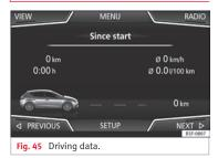
The onboard computer is equipped with 3 memories that work automatically. In these memories you can see the distance travelled, average speed, time passed, average consumption and autonomy of the vehicle.
