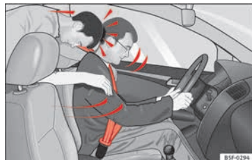
Fig. 87 The unbelted rear passenger is thrown forward violently, hitting the driver wearing a seat belt
