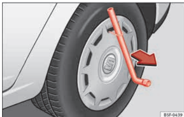
Fig. 66 Removing the full hubcap
