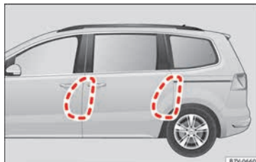
Fig. 32 Range of action of the front and rear side airbags. With 5 and 7 seats.
