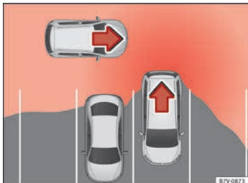
Fig. 225 Schematic representation of the parking assistant: monitored zone around the vehicle being parked.
