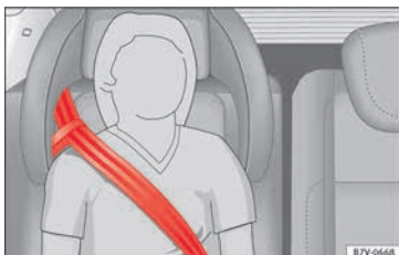
Fig. 97 Integrated child seats. seat belt routing with guide handle
