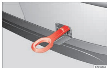
Fig. 105 On the rear bumper, to the right hand side: Towline anchorage in position
