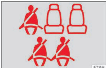
Fig. 84 Example of seat belt status display for the rear seats (here, a 7-seat vehicle) on the instrument panel above, the second row and, below, the third row of seats.
