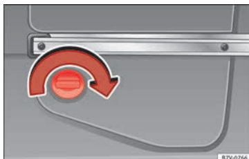
Fig. 237 At the rear left of the luggage compartment: AdBlue tank, behind a cover panel
