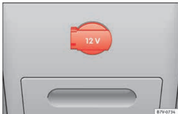
Fig. 194 Centre console, rear section: 12 volt socket
