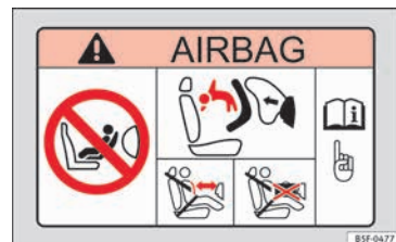
Fig. 35 Passenger's side sun visor: airbag sticker.
