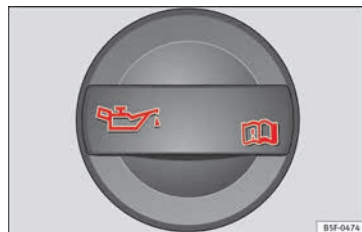
Fig. 56 In the engine compartment: Engine oil filler cap
