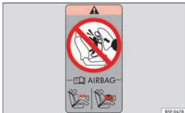
Fig. 36 On the rear frame of the passenger side door: airbag sticker.
