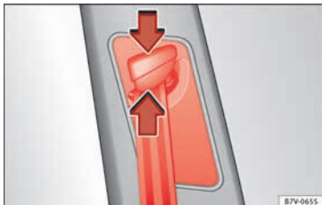
Fig. 91 Next to the front seats: belt height adjuster
