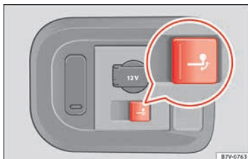
Fig. 230 Right-hand side of the luggage compartment: button to electrically release the tow hitch ball
