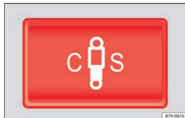
Fig. 228 In the centre console: button for setting the dynamic chassis control.
