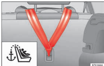
Fig. 39 Upper retaining strap hooked in the luggage compartment
