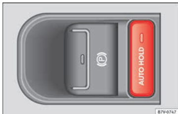
Fig. 207 Detailed view of the centre console: Auto Hold button
