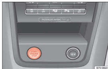
Fig. 200 In the centre console: start-up push button for the Keyless Access lock and start-up system. The layout in right-hand drive vehicles is symmetrical.
