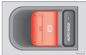
Fig. 202 Detailed view of the centre console: electronic parking brake switch
