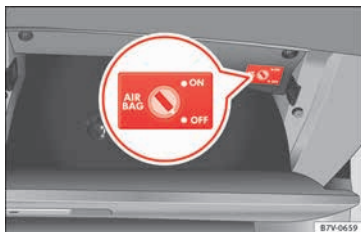
Fig. 28 In the glove compartment on the front passenger side: Key switch for enabling and disabling the front passenger front airbag.
