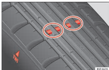
Fig. 253 Tyre tread: tread wear indicators
