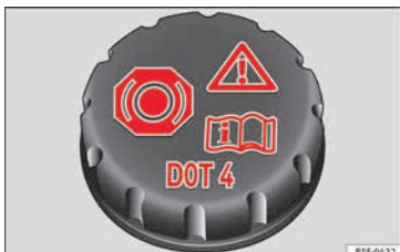
Fig. 58 Engine compartment: brake fluid reservoir cap
