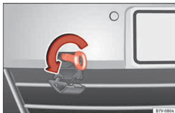
Fig. 73 On the right-hand side of the front bumper: Screw in the towline anchorage.
