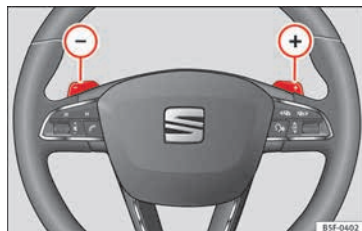
Fig. 205 Steering wheel with two paddle shifts for Tiptronic
