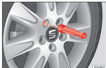
Fig. 72 Changing a wheel: loosen wheel bolts with the socket at the end of the wheel brace
