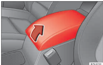
Fig. 123 Front centre armrest: USB/AUX-IN input.
