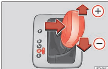
Fig. 204 Selector lever in Tiptronic position (left-hand drive vehicles). The lay-out in right-hand drive vehicles is symmetrically opposed.
