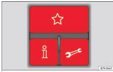
Fig. 124 Three button unit in headliner: controls for the telephone management system.
