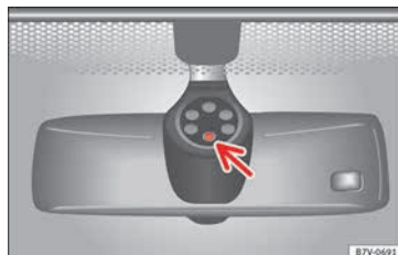
Fig. 146 Rain sensor sensitive surface
