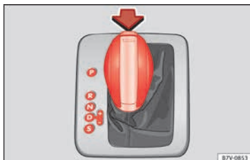
Fig. 49 Automatic gearbox: selector lever positions.
