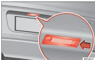
Fig. 116 On the rear bumper: number plate lights
