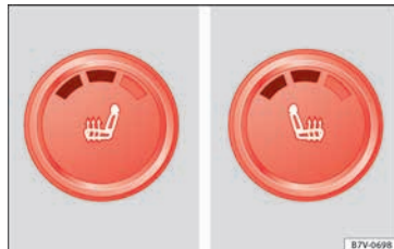
Fig. 155 Detailed view of the centre console: front seat heating controls, here with the second temperature level set
