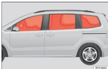
Fig. 34 Deployed head-protection airbags.
