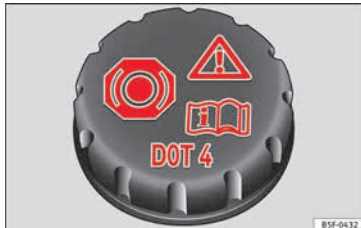
Fig. 247 In the engine compartment: brake fluid reservoir cap
