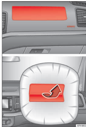
Fig. 27 Location and deployment area of the front airbag for the front passenger
