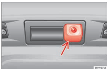
Fig. 215 On the rear lid: location of the rear assist camera
