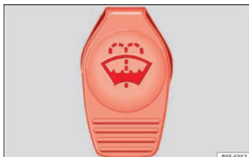
Fig. 59 In the engine compartment: windscreen washer reservoir top.
