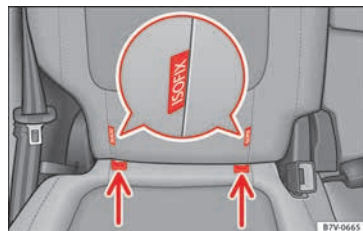
Fig. 38 Version 2: identification of the anchor points for the child seat on the vehicle seat
