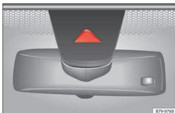
Fig. 220 In the windscreen: field of vision of the lane assist system camera.
