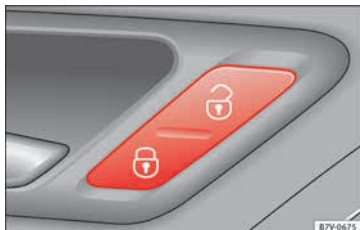
Fig. 131 In the driver door: central locking button
