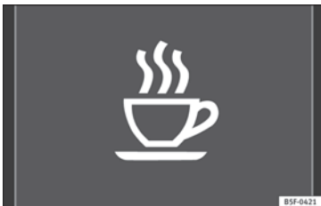
Fig. 227 On the instrument panel display: tiredness detection symbol
