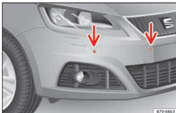
Fig. 210 Parking sensor system sensors on the front bumper
