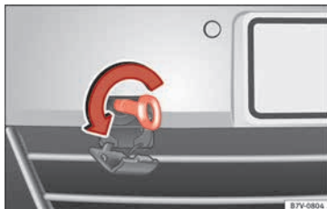
Fig. 104 On the right-hand side of the front bumper: Screw in the towline anchorage.
