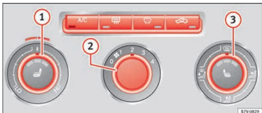
Fig. 52 Detailed view of the centre console: Electronic manual air conditioning controls
