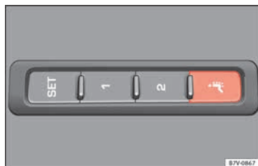
Fig. 157 On the side of the front seat: lumbar massage function switch.
