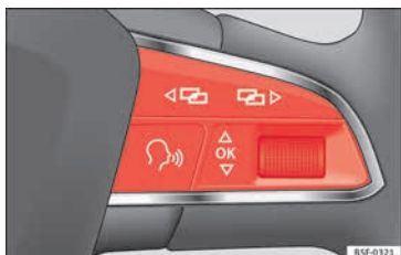
Fig. 46 Multifunction steering wheel: buttons to access the instrument panel menus
