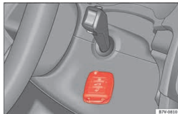
Fig. 201 Emergency ignition in vehicles with KESSY.
