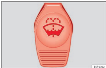
Fig. 247 In the engine compartment: windscreen washer reservoir top
