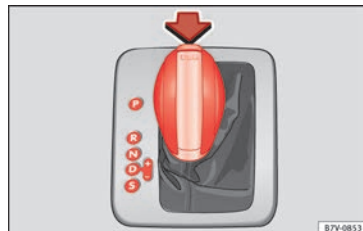
Fig. 202 Automatic gearbox selector lever with locking button (arrow)
