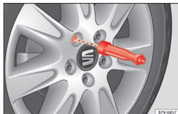
Fig. 71 Changing a wheel: loosen wheel bolts with the socket at the end of the wheel brace
