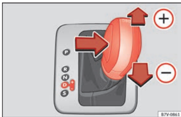
Fig. 203 Selector lever in Tiptronic position (left-hand drive vehicles). The lay-out in right-hand drive vehicles is symmetrically opposed.
