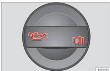
Fig. 242 In the engine compartment: Engine oil filler cap.
