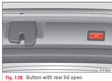
Fig. 138 Button with rear lid open
