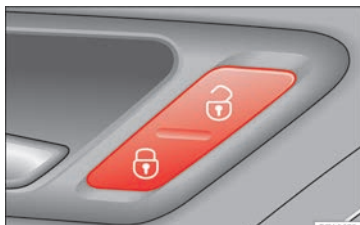
Fig. 2 In the driver door: central locking button
