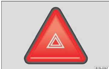
Fig. 140 In the centre of the dash panel: push button for hazard warning lights.
