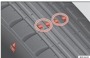
Fig. 252 Tyre tread: tread wear indicators
