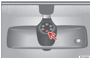
Fig. 145 Rain sensor sensitive surface
