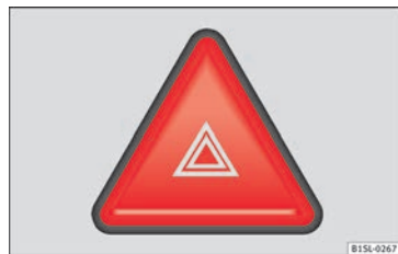
Fig. 42 Dash panel: switch for hazard warning lights.
