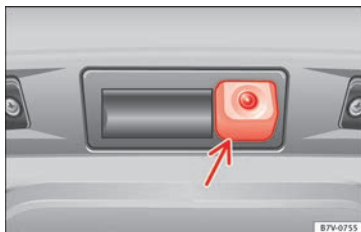
Fig. 214 On the rear lid: location of the rear assist camera
