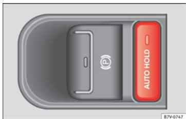
Fig. 206 Detailed view of the centre console: Auto Hold button
