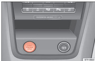
Fig. 199 In the centre console: start-up push button for the Keyless Access lock and start-up system. The layout in right-hand drive vehicles is symmetrical.
