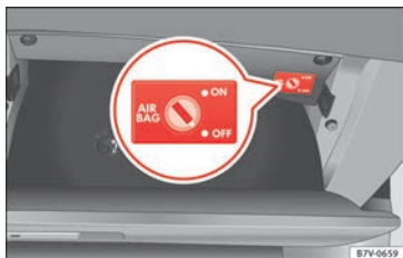
Fig. 27 In the glove compartment on the front passenger side: Key switch for enabling and disabling the front passenger front airbag.
