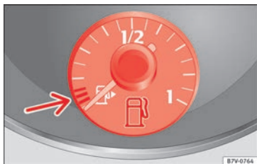
Fig. 234 On the instrument panel: Fuel gauge for petrol and diesel
