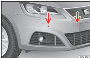
Fig. 209 Parking sensor system sensors on the front bumper
