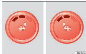
Fig. 154 Detailed view of the centre console: front seat heating controls, here with the second temperature level set
