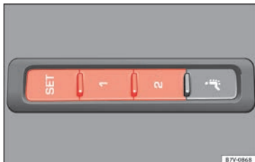
Fig. 157 Memory buttons on the outside of the driver seat
