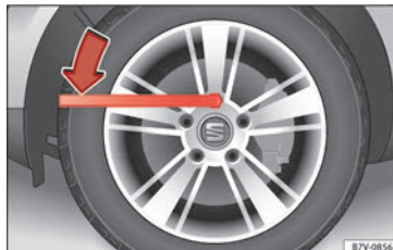
Fig. 67 Changing a wheel: Slacken the wheel bolts.
