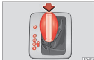
Fig. 48 Automatic gearbox: selector lever positions.
