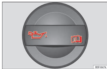
Fig. 55 In the engine compartment: Engine oil filler cap
