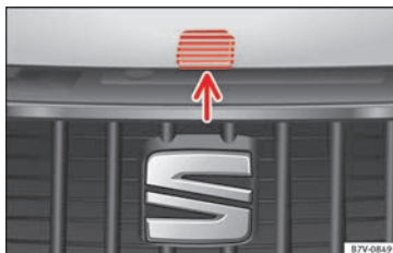
Fig. 239 Release lever to open the bonnet in the radiator grille
