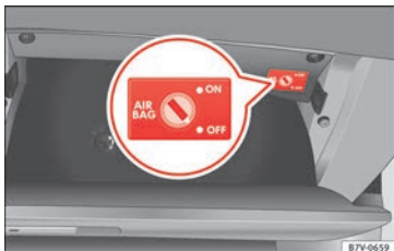
Fig. 92 In the glove compartment on the front passenger side: Key switch for enabling and disabling the front passenger front airbag.
