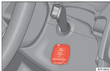
Fig. 200 Emergency ignition in vehicles with Keyless Access.
