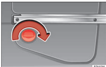
Fig. 236 At the rear left of the luggage compartment: AdBlue tank, behind a cover panel
