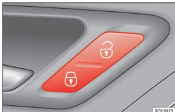
Fig. 130 In the driver door: central locking button
