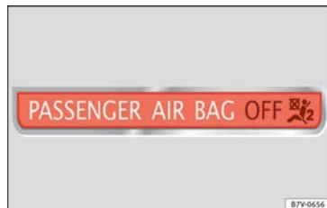
Fig. 91 Control lamp for disabling the front passenger front airbag on the dash panel
