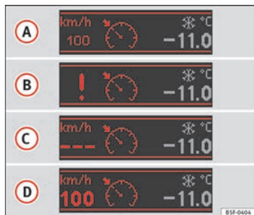
Fig. 218 Instrument panel display: CCS status indications
