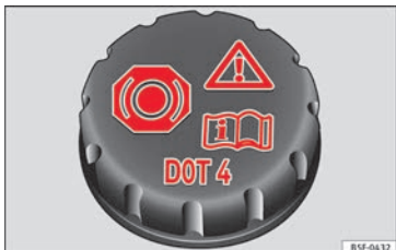
Fig. 57 Engine compartment: brake fluid reservoir cap
