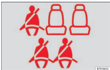
Fig. 83 Example of seat belt status display for the rear seats (here, a 7-seat vehicle) on the instrument panel above, the second row and, below, the third row of seats.
