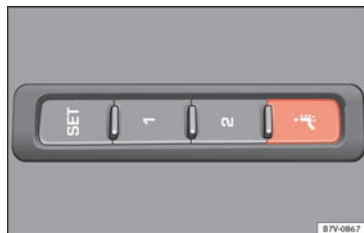
Fig. 156 On the side of the front seat: lumbar massage function switch.
