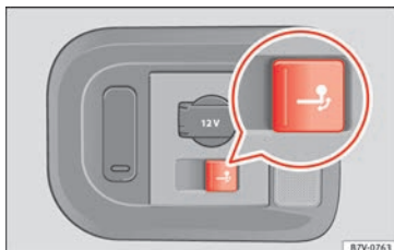
Fig. 229 Right-hand side of the luggage compartment: button to electrically release the tow hitch ball
