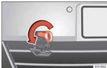
Fig. 103 On the right-hand side of the front bumper: Screw in the towline anchorage.
