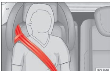
Fig. 96 Integrated child seats. seat belt routing with guide handle
