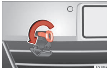
Fig. 72 On the right-hand side of the front bumper: Screw in the towline anchorage.
