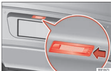
Fig. 115 On the rear bumper: number plate lights
