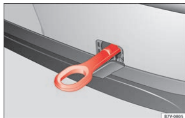
Fig. 104 On the rear bumper, to the right hand side: Towline anchorage in position
