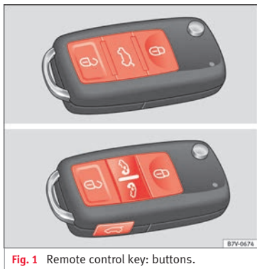
Fig. 1 Remote control key: buttons.
