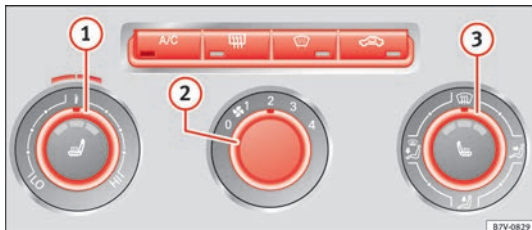
Fig. 51 Detailed view of the centre console: Electronic manual air conditioning controls
