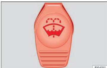
Fig. 58 In the engine compartment: windscreen washer reservoir top.
