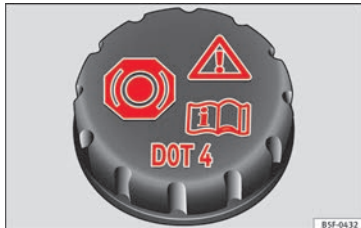
Fig. 246 In the engine compartment: brake fluid reservoir cap
