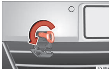
Fig. 71 On the right-hand side of the front bumper: Screw in the towline anchorage.
