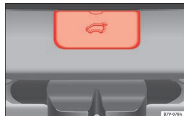
Fig. 8 From the luggage compartment: remove the boot hatch cover.
