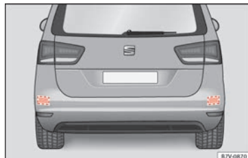
Fig. 222 Rear view of the vehicle: radar sensor zones.
