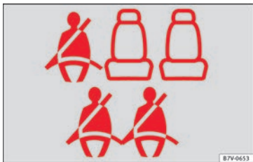
Fig. 82 Example of seat belt status display for the rear seats (here, a 7-seat vehicle) on the instrument panel above, the second row and, below, the third row of seats.
