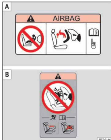
Fig. 35 Airbag stickers - version 2: on the passenger-side sun blind [A] and on the rear frame of the front passenger's door [B].
