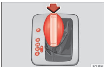
Fig. 201 Automatic gearbox selector lever with locking button (arrow)
