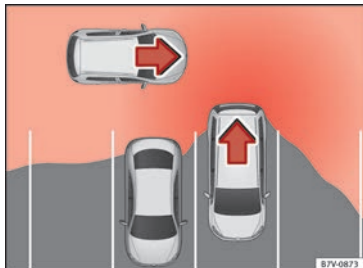
Fig. 225 Schematic representation of the rear cross traffic alert: zone monitored around the vehicle exiting the parking space.
