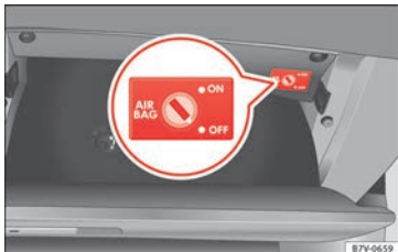
Fig. 91 In the glove compartment on the front passenger side: Key switch for enabling and disabling the front passenger front airbag.
