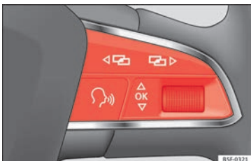
Fig. 45 Multifunction steering wheel: buttons to access the instrument panel menus
