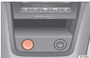
Fig. 198 In the centre console: start-up push button for the Keyless Access lock and start-up system. The layout in right-hand drive vehicles is symmetrical.
