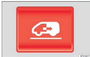
Fig. 134 On the dash panel, on the remote control key and on the interior lining of the sliding door: button for opening and closing the electric sliding door.
