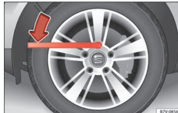
Fig. 66 Changing a wheel: Slacken the wheel bolts.
