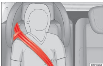
Fig. 95 Integrated child seats. seat belt routing with guide handle
