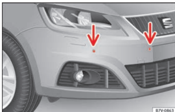
Fig. 208 Parking sensor system sensors on the front bumper
