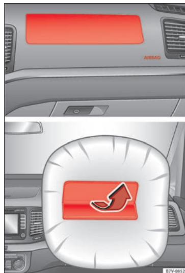
Fig. 26 Location and deployment area of the front airbag for the front passenger
