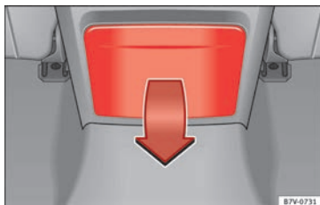
Fig. 189 Centre console, rear section: folding out the drink holder
