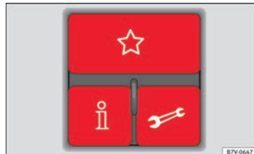
Fig. 122 Three button unit in headliner: controls for the telephone management system.
