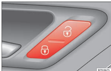
Fig. 129 In the driver door: central locking button
