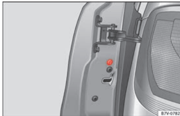
Fig. 4 At the front of the passenger sliding door: Emergency lock, hidden by a rubber cap.
