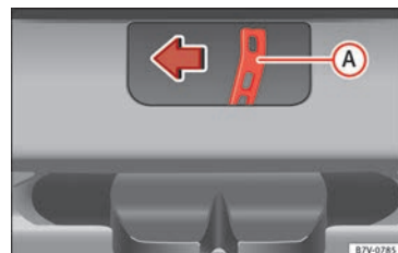
Fig. 9 From the luggage compartment: Emergency unlocking of the boot hatch.
