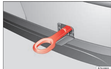
Fig. 72 On the rear bumper, to the right hand side: Towline anchorage in position
