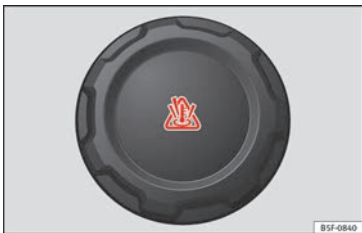
Fig. 55 Engine compartment: coolant expansion tank cap.
