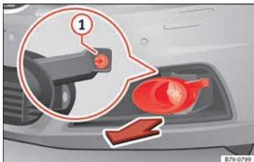
Fig. 108 On the right-hand side of the front bumper: removing the headlights.
