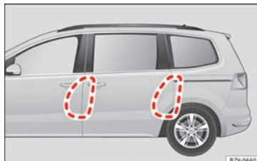
Fig. 31 Range of action of the front and rear side airbags. With 5 and 7 seats.
