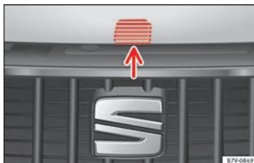
Fig. 240 Release lever to open the bonnet in the radiator grille
