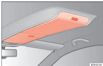
Fig. 175 On the roof console: storage compartment
