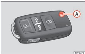
Fig. 124 Vehicle key for vehicles with electric sliding doors
