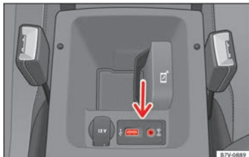
Fig. 120 Front centre armrest: USB/AUX-IN input.
