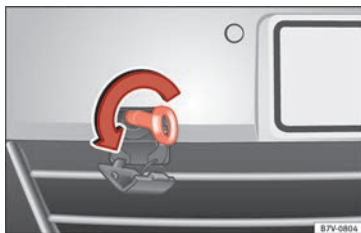
Fig. 102 On the right-hand side of the front bumper: Screw in the towline anchorage.
