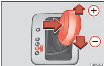
Fig. 202 Selector lever in Tiptronic position (left-hand drive vehicles). The lay-out in right-hand drive vehicles is symmetrically opposed.
