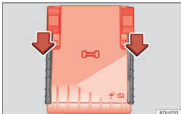
Fig. 59 In the engine compartment: fuse box cover.
