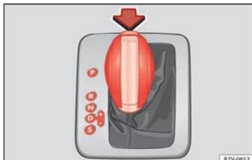
Fig. 48 Automatic gearbox: selector lever positions.
