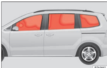
Fig. 33 Deployed head-protection airbags.
