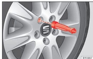
Fig. 70 Changing a wheel: loosen wheel bolts with the socket at the end of the wheel brace
