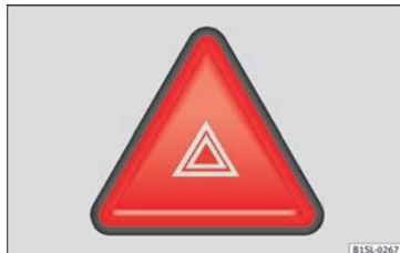
Fig. 139 In the centre of the dash panel: push button for hazard warning lights.
