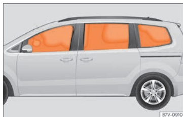
Fig. 35 Deployed head-protection airbags.
