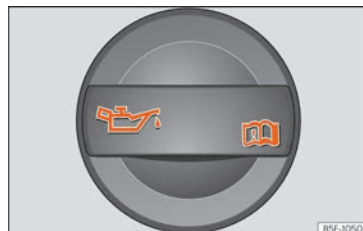
Fig. 292 In the engine compartment: engine oil filler cap.
