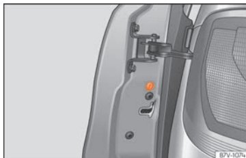
Fig. 6 On the front part of the sliding door: emergency locking, hidden behind a rubber gasket.
