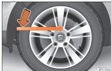
Fig. 69 Tyre change: slacken the wheel bolts.
