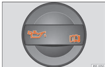
Fig. 57 In the engine compartment: Engine oil filler cap.
