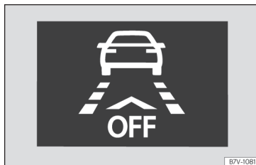
Fig. 260 On the screen of the instrument panel Front Assist switched off message.
