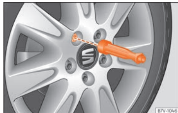
Fig. 73 Changing the tyre: loosen wheel bolts with the socket at the end of the wheel brace
