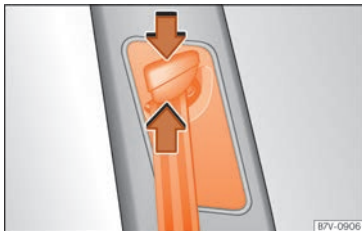
Fig. 92 Near the front seats: seat belt height regulator.
