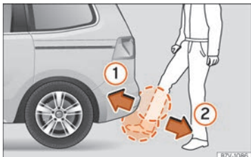
Fig. 142 Rear lid with sensor-controlled opening (Easy Open).
