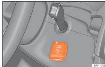
Fig. 238 Emergency ignition in vehicles with Keyless Access.
