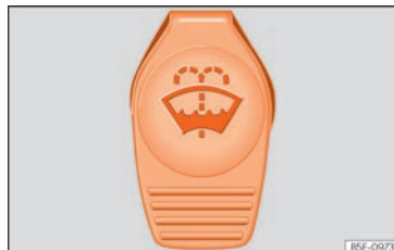
Fig. 60 In the engine compartment: cap of the windscreen washer tank.
