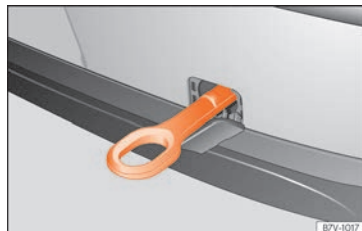
Fig. 75 On the rear bumper, to the right hand side: Towline anchorage in position
