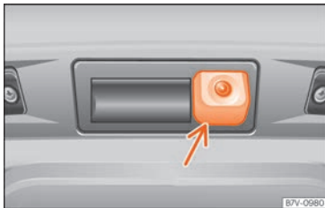
Fig. 253 On the rear lid: location of the rear assist camera.
