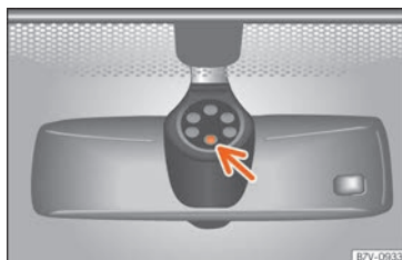
Fig. 149 Rain sensor sensitive surface
