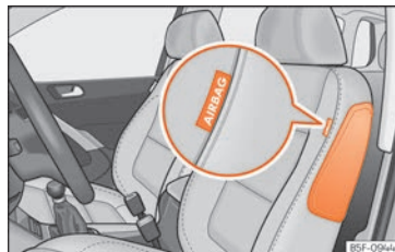
Fig. 32 On the front seat side: location of side airbag.
