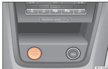
Fig. 237 In the centre console: start-up push button for the Keyless Access lock and start-up system. The layout in right-hand drive vehicles is symmetrical.
