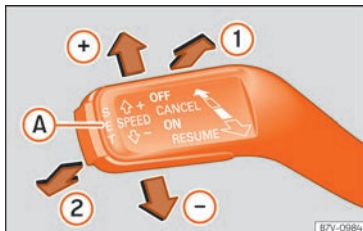
Fig. 49 Left of the steering column: CCS switch and controls.
