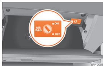
Fig. 29 In the glove box on the passenger side: switch to activate and deactivate the front passenger airbag.
