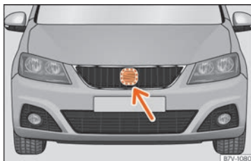
Fig. 259 On the front behind the SEAT badge: radar sensor.
