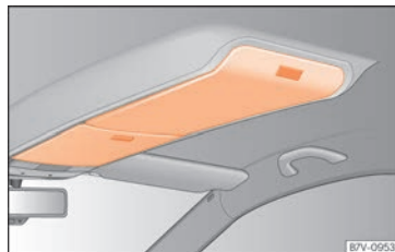
Fig. 180 On the roof console: storage compartment.
