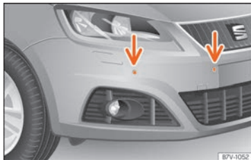
Fig. 247 Parking sensor system sensors on the front bumper
