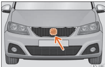
Fig. 263 On the front behind the SEAT badge: radar sensor.
