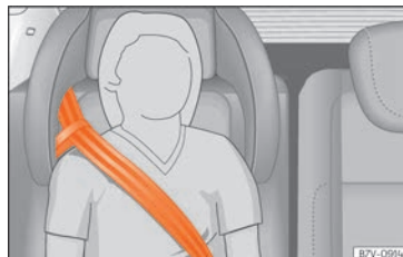
Fig. 98 Embedded child seat: seat belt routing with guide handle. »
