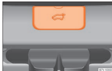
Fig. 10 From the trunk: remove the rear lid.
