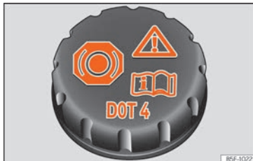
Fig. 296 Engine compartment: brake fluid reservoir cap.
