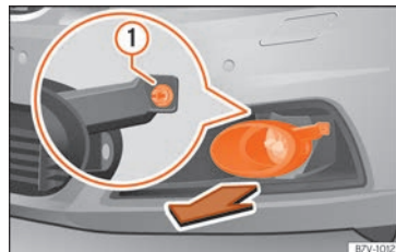
Fig. 111 On the right side of the front bumper: detaching the headlights.
