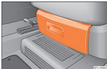
Fig. 188 Drawer under the front seat
