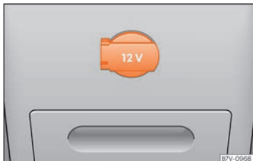
Fig. 197 Centre console, rear section: 12-volt power socket.
