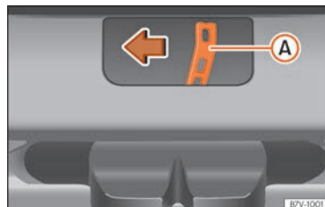
Fig. 11 From the trunk: emergency unlocking of the rear lid.
