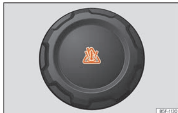
Fig. 58 Engine compartment: coolant expansion tank cap.
