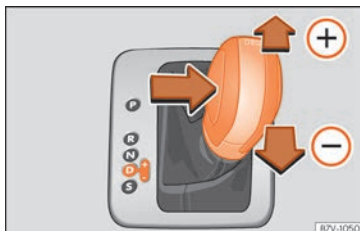
Fig. 239 Selector lever in Tiptronic position (left-hand drive vehicles). The lay-out in right-hand drive vehicles is symmetrically opposed.
