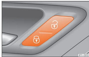
Fig. 90 Driver's door: central locking switch.
