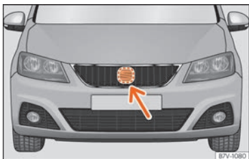
Fig. 244 On the front bumper: radar sensors.
