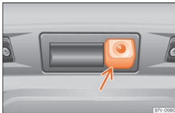
Fig. 249 In the rear bumper: location of the reverse assist camera.
