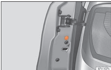
Fig. 96 On the front of the sliding door: emergency lock, hidden by a rubber seal.
