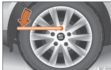
Fig. 45 Wheel change: loosen the wheel nuts.
