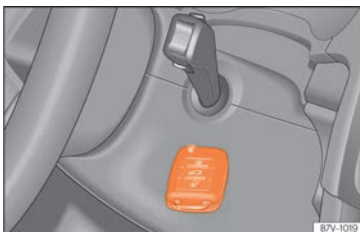
Fig. 235 Emergency ignition in vehicles with Keyless Access.
