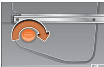
Fig. 283 On the rear left side of the luggage compartment: AdBlue tank, behind a cover.
