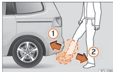
Fig. 106 Rear lid with sensor-controlled opening (Easy Open).
