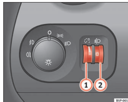
Fig. 77 Detail of the dash panel: Regulation for instrument and switch illumination and headlight range control
