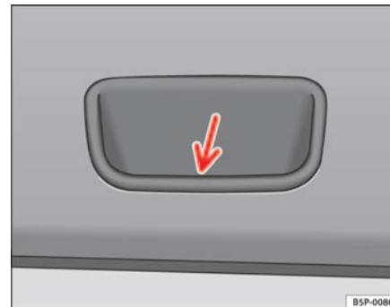
Fig. 69 Detail of the tailgate inner trim: recessed handle for closing the tailgate
