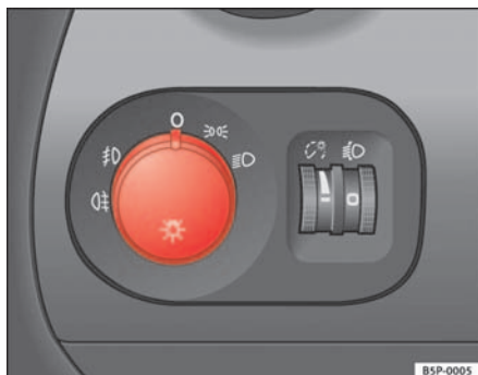
Fig. 75 Detail of the dash panel: Switch for lights, fog lights and rear fog light
