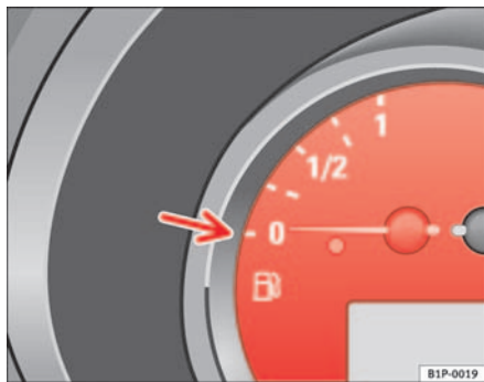
Fig. 34 Details of the instrument panel: Fuel gauge
