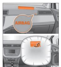
Fig. 23 Front passenger airbag located in dash panel.
