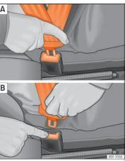
**Fig. 92** Positioning and removing the seat belt buckle.
