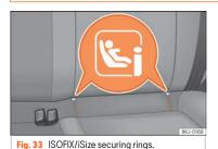
Child seats can be secured quickly, easily and safely on the rear outer seats with the "ISOFIX" and Top Tether\* sustem.
