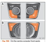
heating switch A: version with Climatronic. B: version with manual air conditioning.
