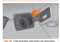
The tank flap is released electronically by means of the central locking and is located at the rear of the vehicle, on the right. The tank holds approximately 40 litres.
