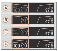
**Fig. 226** Instrument panel display: CCS status indications.
