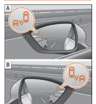
Fig. 242 On external rear-view mirrors: blind spot detector display.
