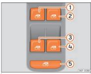
Fig. 141 Detail of the driver door: controls for the front and rear windows.
