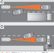
Fig. 241 (C) Vehicle changing lanes. (D) One vehicle turning and another stationary.
