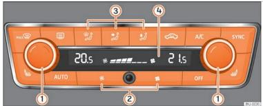
**Fig. 55** In the centre console: Climatronic control panel.
