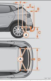
Fig. 276 Attachment points for towing bracket.
