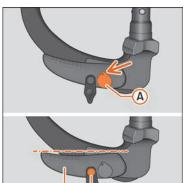
Fig. 266 Reserve position: position of the lever and the release bolt.
