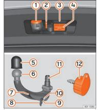
Fig. 263 Towing bracket device support / detachable ball joint / key.
