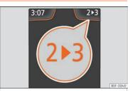
Fig. 223 Instrument panel: gear-change indicator (manual gearbox).
