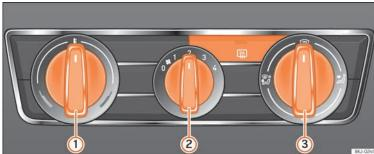
Fig. 169 Heating controls on the dash panel.
