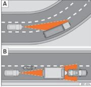
Fig. 240 (A) Vehicle on a bend. (B) Motorcyclist ahead out of range of the radar sensor.
