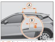
**Fig. 167** Attachment points for the roof railings for the roof carrier system.
