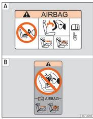
Fig. 30 Airbag adhesives - version 1: on the passenger-side sun blind A and on the rear frame of the front passenger's door B.
