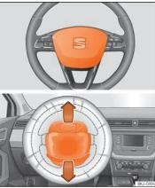
Fig. 22 Driver airbag located in steering wheel.
