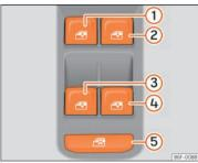
Fig. 13 Detail of the driver door: controls for the windows.
