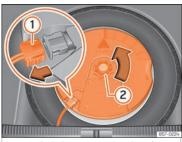
Fig. 287 In the boot: remove the subwoofer.
