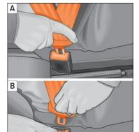
Fig. 17 Positioning and removing the seat belt buckle
