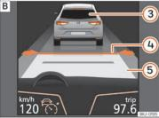
Fig. 235 On the instrument panel display: (A) ACC inactive (Standby). (B) ACC active.
