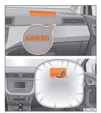
**Fig. 15** Front passenger airbag located in dash panel.
