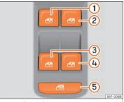
Fig. 96 Detail of the driver's door: window controls.
