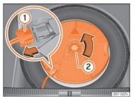
Fig. 210 In the luggage compartment: remove the subwoofer
