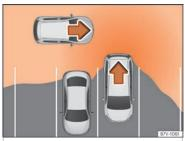
Fig. 167 Schematic representation of the rear cross traffic alert assistant: zone monitored around the vehicle while leaving a parking space.
