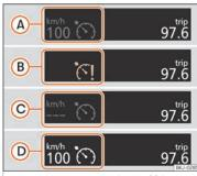
**Fig. 150** Instrument panel display: GRA status indications.
