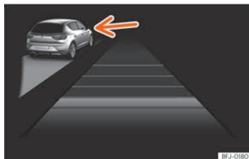
Fig. 161 On the instrument panel display: ACC active, vehicle detected in an outer lane.
