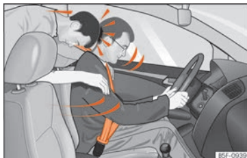
Fig. 9 The unbelted passenger in the rear seat is thrown forward violently, hitting the driver who is wearing a seat belt.
