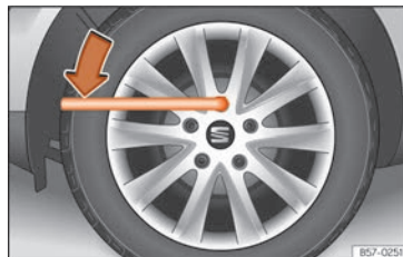
Fig. 35 Wheel change: loosen the wheel nuts.
