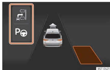
Fig. 170 On the instrument panel display: view of the parking assist system with reduced view.
