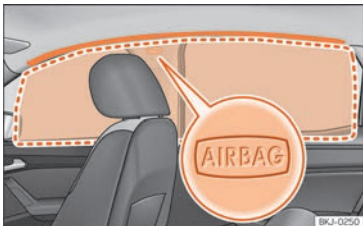
Fig. 20 Location and deployment area of the head-protection airbag.
