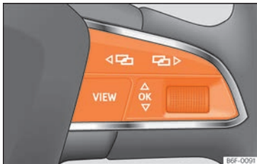
Fig. 74 Right side of the multifunction steering wheel: buttons to the menus and information displays on the instrument panel.
