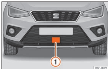
Fig. 145 On the front bumper: radar sensors.
