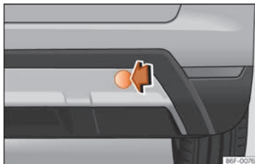
Fig. 46 On the right side of the rear bumper: remove the cover.
