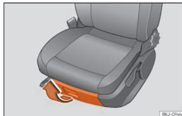
Fig. 115 Storage compartment under the right front passenger seat.
