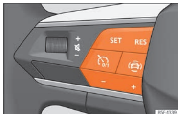
Fig. 145 On the multifunction steering wheel: buttons to operate the speed limiter.
