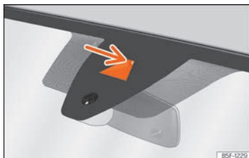
Fig. 141 On the windscreen: field of vision of the Lane Assist system.
