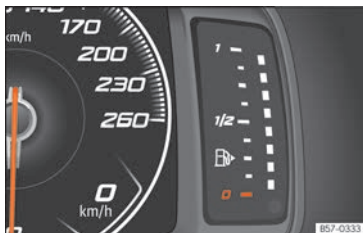
Fig. 66 Digital instrument panel: fuel gauge.
