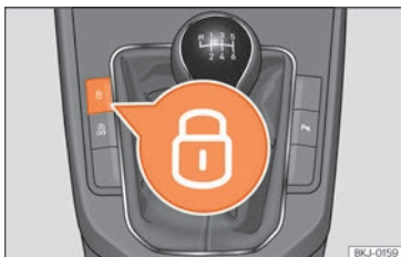
Fig. 82 Centre console: central locking button.
