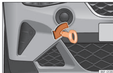
Fig. 45 Right side of the front bumper: towline anchorage in position.
