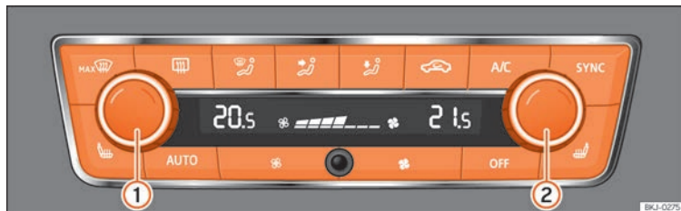
Fig.119 In the centre console: Climatronic controls.
