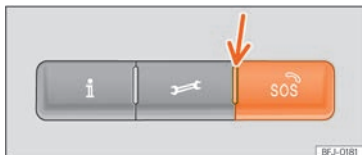
Fig. 29 On the roof console: voice service controls
