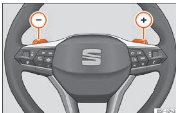
Fig. 136 Steering wheel: automatic transmission levers
