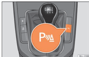
Fig. 170 Centre console: parking aid button [depending on the version].
