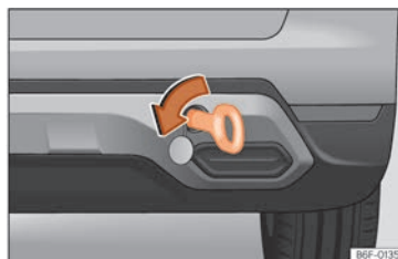
Fig. 47 On the right side of the rear bumper: towline anchorage in position.
