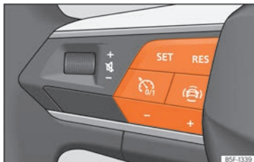
Fig. 146 On the multifunction steering wheel: buttons to operate the speed limiter.
