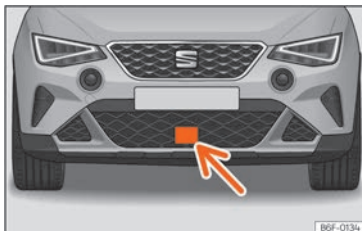
Fig. 139 On the front bumper: radar sensors.
