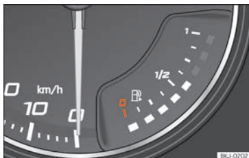
Fig. 65 Analogue instrument panel: fuel gauge
