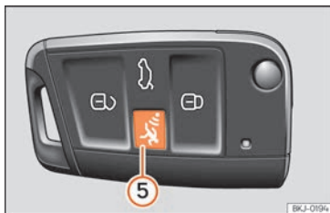
Fig. 78 Vehicle key with alarm button.
