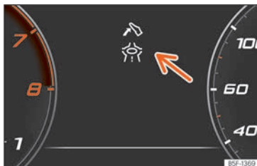
Fig. 64 Eco-efficient driving assistance indication (schematic representation).
