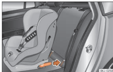
Fig. 25 Rear seats: fitting a child seat with the ISOFIX system.
