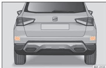
Fig. 98 Rear view of the vehicle: radar sensor areas.
