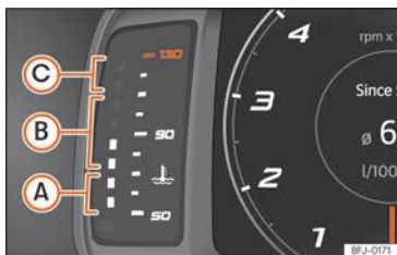
Fig. 9 SEAT Digital Cockpit digital instrument cluster: engine coolant temperature indicator.
