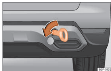
Fig. 167 Right side of the rear bumper: towline anchorage screwed in.
