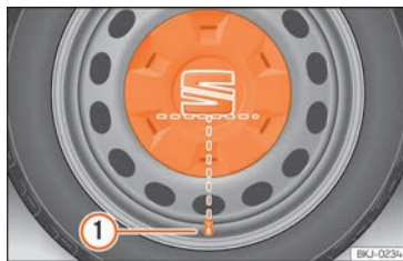
Fig. 193 Correct positioning of the central wheel trim for steel rims.
