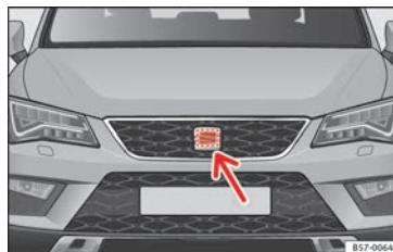
Fig. 196 On the front behind the SEAT badge: radar sensor.
