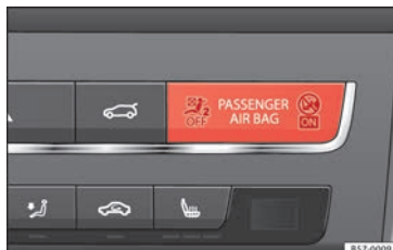
Fig. 23 Dash panel: control lamp for deactivated front passenger airbag in centre console.
