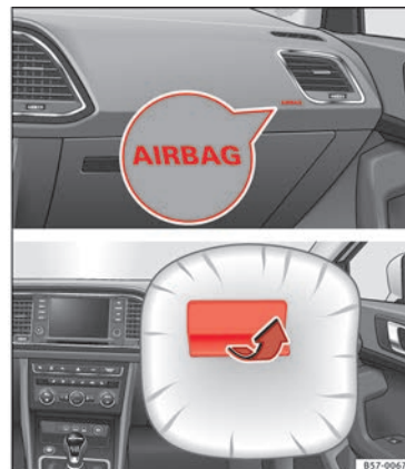
Fig. 21 Front passenger airbag located in dash panel.
