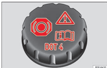
Fig. 64 Engine compartment: brake fluid reservoir cap.
