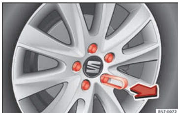
Fig. 72 Wheel: wheel bolts with caps.
