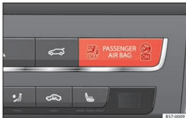
Fig. 96 Dash panel: control lamp for deactivated front passenger airbag in centre console.
