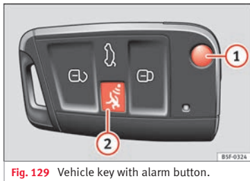
Fig. 129 Vehicle key with alarm button.
