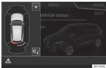
Fig. 225 Miniature indication of automatic activation.
