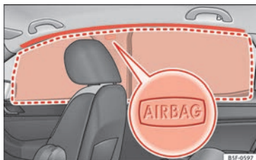
Fig. 28 Location of head-protection airbags.
