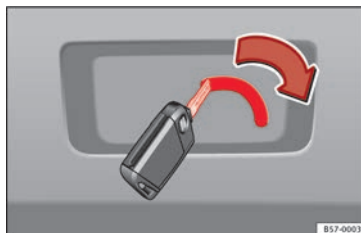
Fig. 8 Luggage compartment: emergency release.
