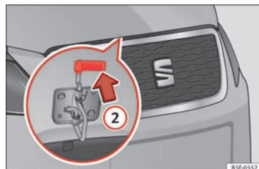
Fig. 10 Cam under the bonnet
