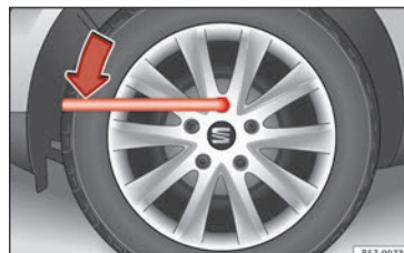
Fig. 74 Wheel: loosen the wheel bolts.
