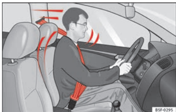
Fig. 90 Drivers with properly worn seat belts will not be thrown forward in the event of sudden braking.
