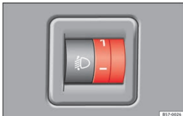
Fig. 145 Next to the steering wheel: Headlight range control
