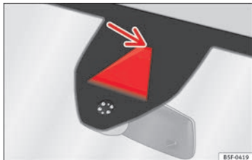
Fig. 202 In the windscreen: field of vision of the Lane Assist system camera.
