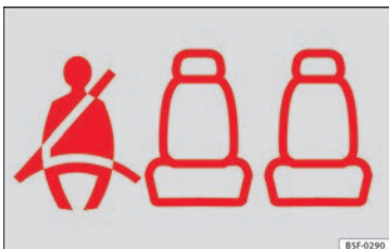
Fig. 89 Instrument panel: right rear seat occupied and corresponding seat belt fastened display.
