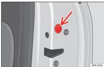
Fig. 4 Locking the door manually.
