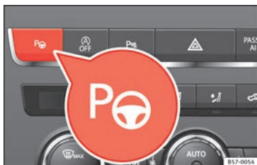
Fig. 217 At the top of the centre console: button to switch on the Park Assist system.
