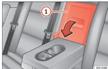
Fig. 163 On the rear seat backrest: opening the tailboard.
