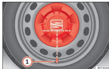
Fig. 71 Correct positioning of the central wheel trim for steel rims.
