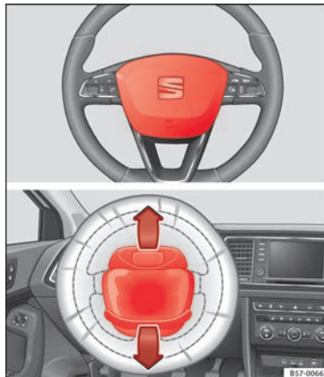
Fig. 20 Driver airbag located in steering wheel.
