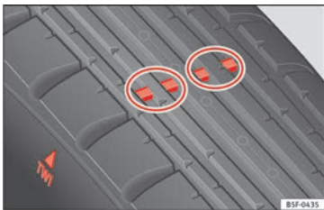
Fig. 243 Tyre tread: tread wear indicators
