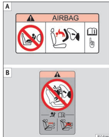
Fig. 30 Airbag stickers - version 2: on the passenger-side sun blind A and on the rear frame of the front passenger's door B .
