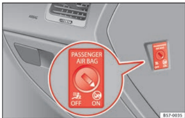
Fig. 95 Switch for activating and deactivating the front passenger airbag.
