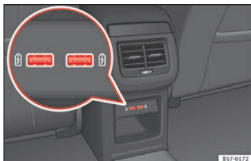
Fig. 125 Centre console, rear section: USB connectors.
