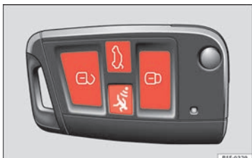
Fig. 1 Remote control key: buttons.
