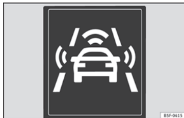
Fig. 190 On the instrument panel display: pre-warning messages.
