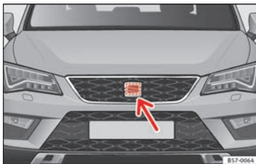
Fig. 191 On the front behind the SEAT badge: radar sensor.
