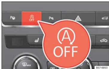
Fig. 184 Centre console: Start-Stop system button.
