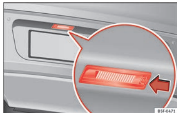
Fig. 115 In the rear bumper: number plate light.
