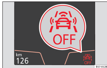
Fig. 192 On the instrument panel display: Front Assist switched off message.
