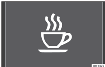
Fig. 215 On the instrument panel display: fatigue detection symbol.
