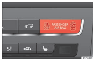
Fig. 53 Warning lamp for disabling the front passenger airbag.
