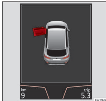
Fig. 52 On the instrument panel display: door open.
