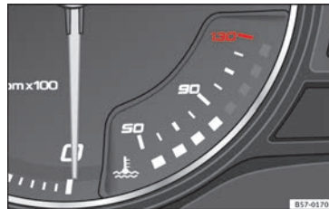
Fig. 121 Instrument panel: coolant temperature gauge
