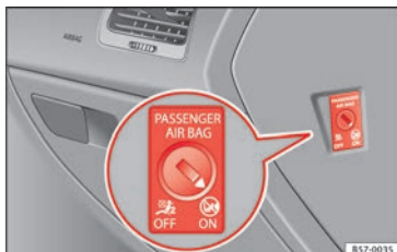
Fig. 22 Front passenger front airbag switch.
