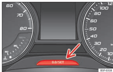
Fig. 120 Instrument panel: odometer and reset button.
