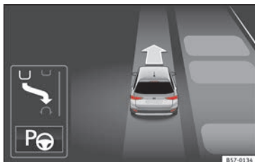
Fig. 219 On the instrument panel display: displaying the Park Assist system with reduced display.
