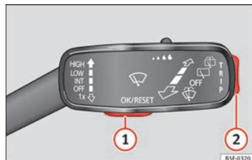
Fig. 43 Windscreen wiper lever: control buttons.
