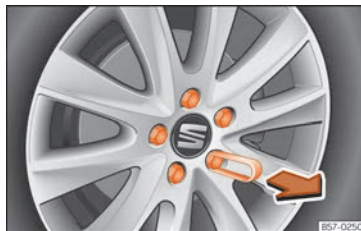
Fig. 75 Wheel: wheel bolts with caps.
