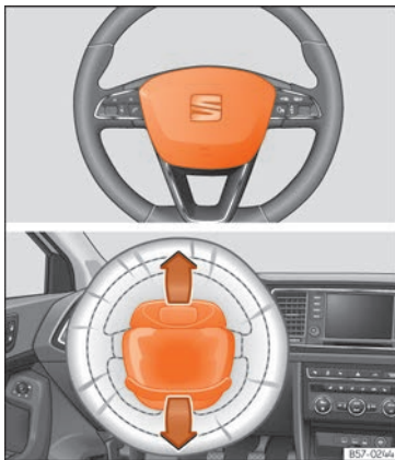
Fig. 26 Driver airbag located in steering wheel.
