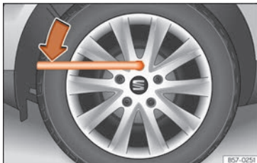
Fig. 77 Wheel: loosen the wheel bolts.
