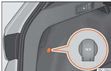
Fig. 169 Detailed view of the side trim in the boot: 12-volt power socket.
