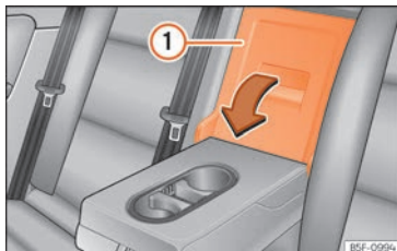
Fig. 174 On the rear seat backrest: opening the tailboard.
