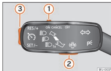
Fig. 54 Left of the steering column: CCS switch and controls.
