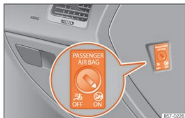
Fig. 28 Front passenger front airbag switch.
