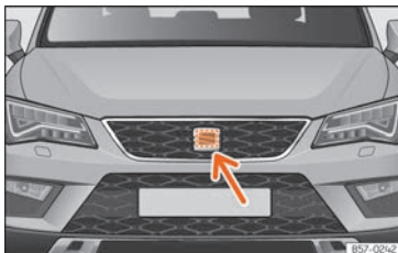
Fig. 255 On the front behind the SEAT badge: radar sensor.
