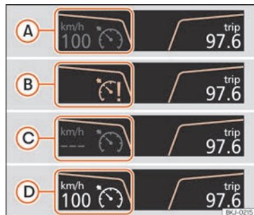
Fig. 250 Instrument panel display: CCS status indications.
