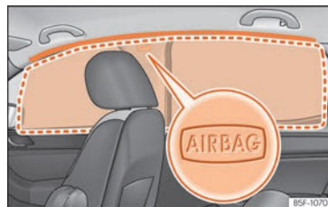
Fig. 34 Location of head-protection airbags.
