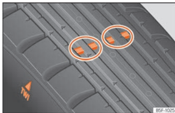
Fig. 307 Tyre profile: tread wear indicators.
