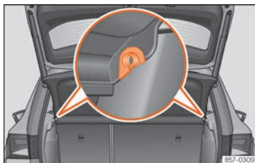
Fig. 171 In the boot: removing and installing the shelf.
