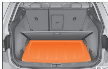
Fig. 173 In the boot: fitting the rear shelf.
