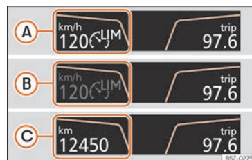
Fig. 251 On the instrument panel display: indications of the speed limiter status.
