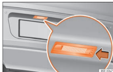
Fig. 118 In the rear bumper: number plate light.
