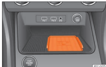
Fig. 239 Centre console: slot for mobile phone connection.
