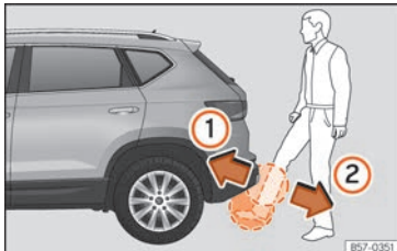
Fig. 103 Rear lid with sensor-controlled opening [Easy Open].
