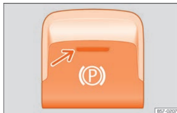
Fig. 279 In the lower part of the centre console: electronic parking brake button
