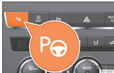
Fig. 282 In the upper part of the centre console: button to switch on the Park Assist system.
