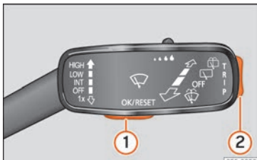
Fig. 79 Wiper lever: control keys.
