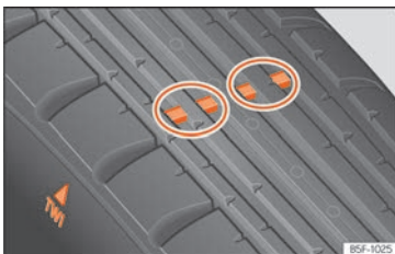
Fig. 318 Tyre profile: tread wear indicators.
