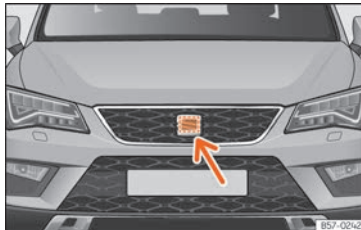
Fig. 263 On the front behind the SEAT badge: radar sensors.
