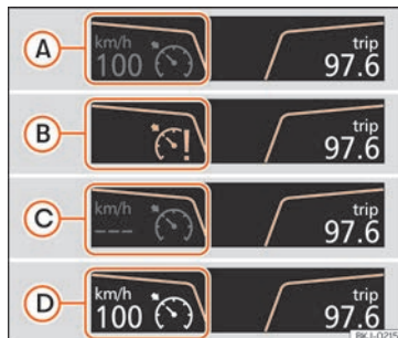
Fig. 251 Instrument panel display: GRA status indications.
