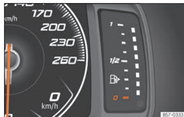
Fig.76 Digital instrument panel: fuel gauge. »
