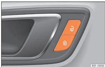
Fig. 92 Driver's door: central locking switch.
