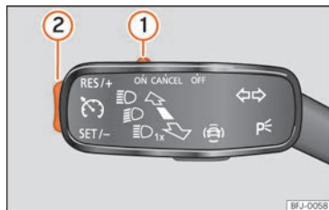
Fig. 252 On the turn signal lever: controls for operating the GRA.
