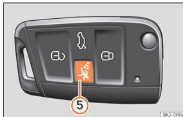
Fig. 88 Vehicle key with alarm button.
