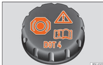
Fig. 315 Engine compartment: brake fluid reservoir cap.
