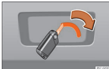
Fig. 105 Detail of the luggage compartment: emergency unlocking
