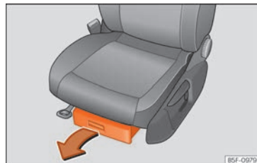
Fig. 148 Storage compartment under the front seats.
