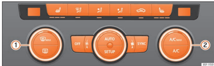
Fig. 153 In the centre console: Climatronic controls.
