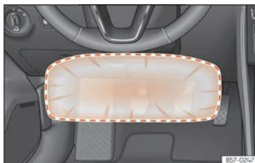
Fig. 20 On the driver side: airbag action radius for the knees.
