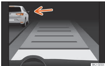
Fig. 266 On the instrument panel display: ACC active, vehicle detected in an outer lane.
