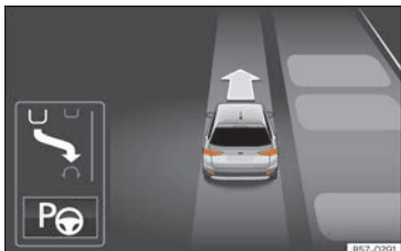
Fig. 283 On the instrument panel display: view of the parking assist system with reduced view.
