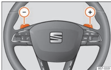
Fig. 245 Steering wheel: automatic transmission levers
