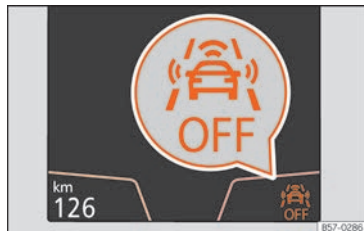
Fig. 258 On the instrument panel display: Front Assist deactivated indication.
