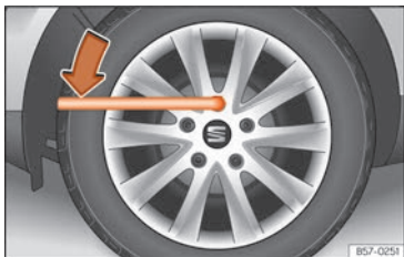
Fig. 38 Wheel change: loosen the wheel nuts.
