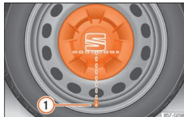
Fig. 35 Correct positioning of the central wheel trim for steel rims.
