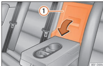
Fig. 142 In the rear seat backrest: opening the trapdoor.
