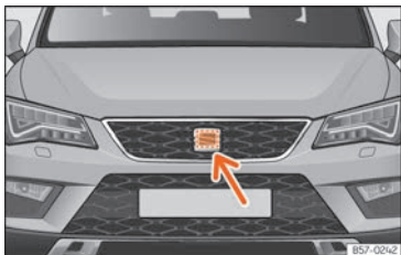
Fig. 257 On the front behind the SEAT badge: radar sensors.
