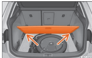
Fig. 137 Variable luggage compartment floor: inclined position.
