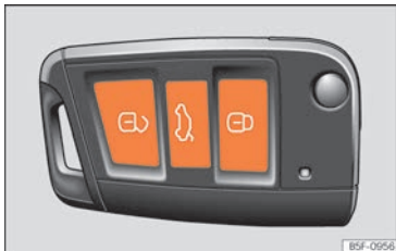
Fig. 91 Remote control key: buttons.
