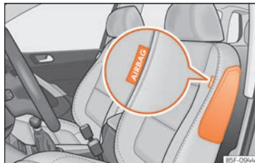
Fig. 21 Side airbag in driver's seat.
