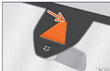
Fig. 269 On the windscreen: field of vision of the Lane Assist system.
