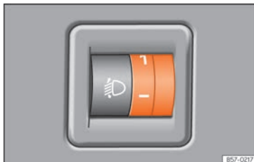
Fig. 116 Next to the steering wheel: headlight range control.
