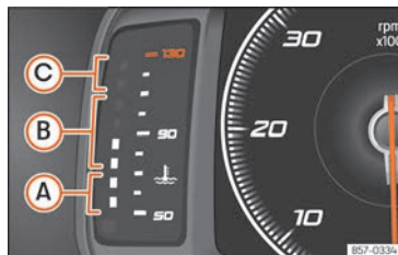
Fig. 78 Digital instrument panel: engine coolant temperature indicator.
