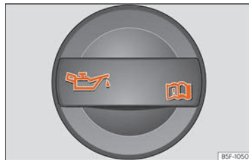
Fig. 312 In the engine compartment: Engine oil filler cap. »
