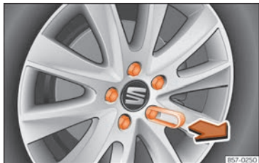
Fig. 36 Wheel: wheel nuts with caps.
