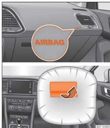
Fig. 16 Front passenger airbag located in dash panel.
