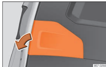
Fig. 63 Rear lid open: remove the cover.
