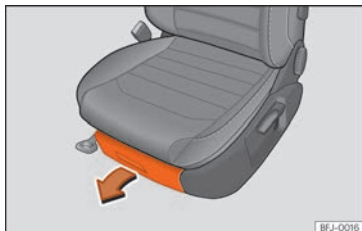
Fig. 141 Drawer under the front seat
