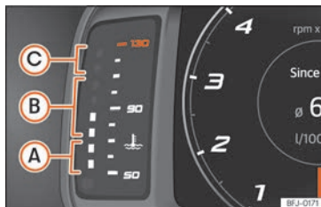
Fig. 74 Digital instrument panel: engine coolant temperature indicator.
