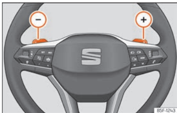
Fig. 164 Steering wheel: automatic transmission levers
