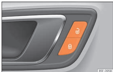
Fig. 90 Driver's door: central locking switch.
