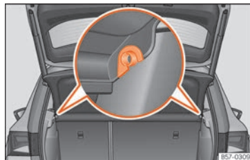
Fig. 127 In the luggage compartment: removing and fitting the shelf.
