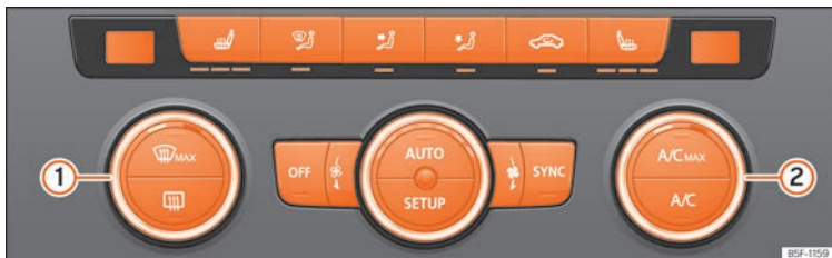
Fig. 145 In the centre console: Climatronic controls.
