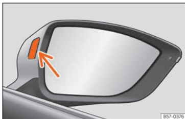
Fig. 190 Control lamp of the lane departure warning.
