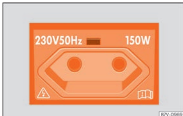
Fig. 144 On the left side of the luggage compartment: 230 volt power socket.
