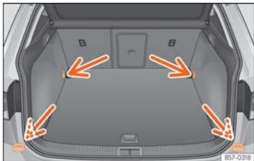
Fig. 132 In the luggage compartment: fastening rings.
