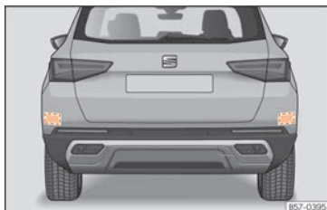
Fig. 170 Rear view of the vehicle: radar sensor zones.
