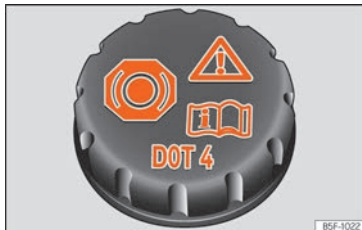
Fig. 226 Engine compartment: brake fluid reservoir cap.
