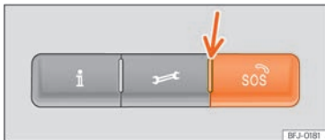
Fig. 30 On the roof console: voice service controls
