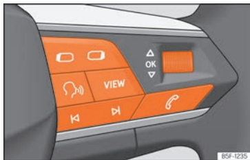
Fig. 75 Right side of the multifunction steering wheel: buttons to the menus and information displays on the instrument panel.
