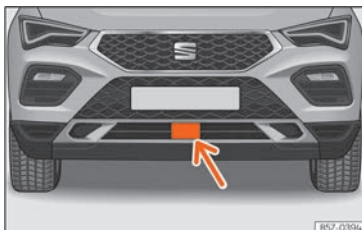
Fig. 167 On the front bumper: radar sensors.
