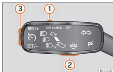
Fig. 176 On the turn signal lever: buttons to operate the speed limiter.
