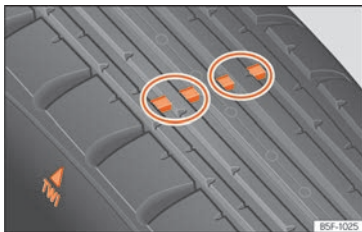
Fig. 230 Tyre profile: tread wear indicators.
