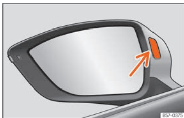
Fig. 189 Control lamp of the lane departure warning.
