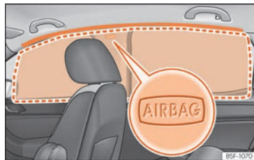
Fig. 22 Location of head-protection airbags.
