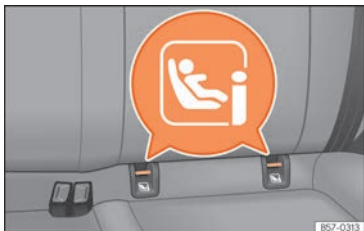
Fig. 26 Rear seat: ISOFIX/i-Size securing rings.
