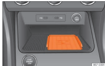
Fig. 154 In the centre console: pad for the mobile phone connection.
