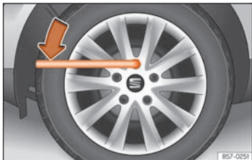
Fig. 36 Wheel change: loosen the wheel nuts.
