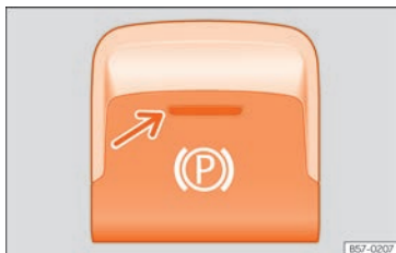
Fig. 194 In the lower part of the centre console: electronic parking brake button
