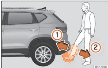
Fig. 100 Rear lid with sensor-controlled opening [Easy Open].
