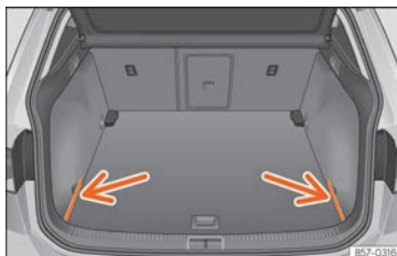
Fig. 128 In the luggage compartment: covers for storing the rear shelf.
