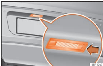
Fig. 63 In the rear bumper: Number plate light.
