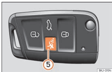
Fig. 86 Vehicle key with alarm button.
