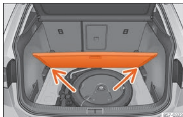
Fig. 131 Variable luggage compartment floor: inclined position.
