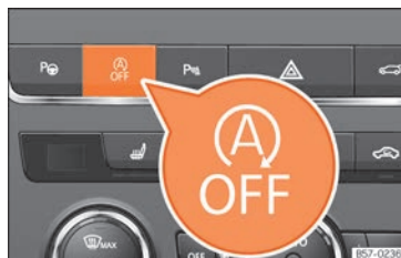
Fig. 160 Centre console: Start-stop system button.
