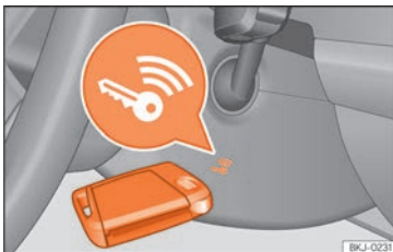
Fig. 159 On the right of the steering column: emergency start.
