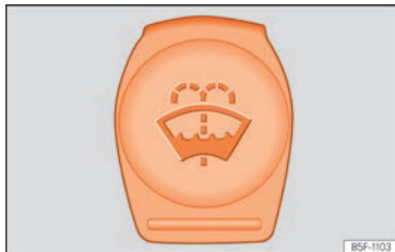
Fig. 227 In the engine compartment: window washer tank cap.
