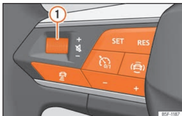
Fig. 83 Controls on the steering wheel.
