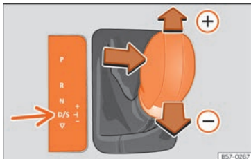
Fig. 163 Lever in the Tiptronic position
