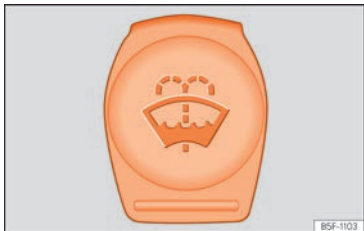
Fig. 217 In the engine compartment: window washer tank cap.
