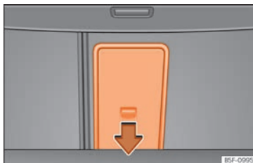
Fig. 126 In the luggage compartment: opening the trapdoor.
