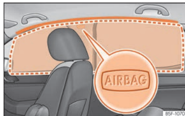
Fig. 22 Location of head-protection airbags.
