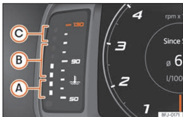
Fig. 62 Digital instrument panel: engine coolant temperature indicator.
