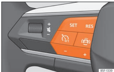
Fig. 163 On the multifunction steering wheel: buttons to operate the speed limiter.
