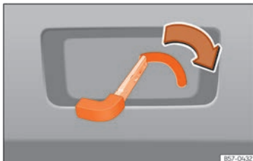
Fig. 91 Detail of the luggage compartment: emergency unlocking
