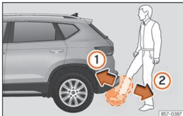
Fig. 89 Rear lid with sensor-controlled opening (Easy Open).
