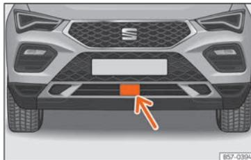
Fig. 157 On the front bumper: radar sensors.
