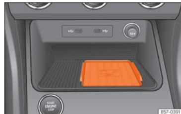
Fig. 145 In the centre console: pad for the mobile phone connection.
