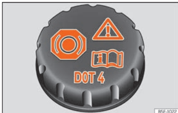
Fig. 216 Engine compartment: brake fluid reservoir cap.
