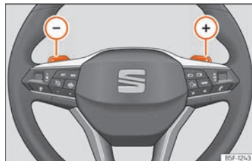
Fig. 154 Steering wheel: automatic transmission levers
