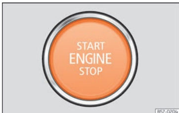
Fig. 148 In the lower part of the centre console: start button.
