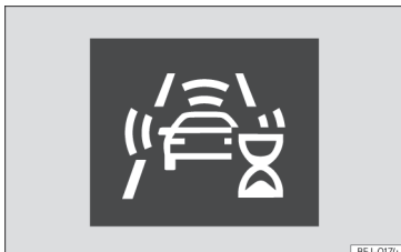
Fig. 167 On the instrument panel display: initial system self-calibration indication.
