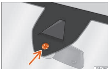
Fig. 103 Rain sensor sensitive surface
