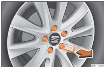
Fig. 34 Wheel: wheel nuts with caps.
