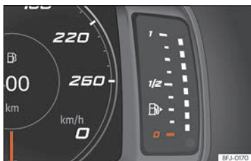
Fig. 60 Digital instrument panel: fuel gauge.
