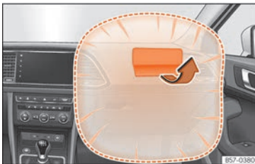
Fig. 15 Front passenger airbag located in dash panel.
