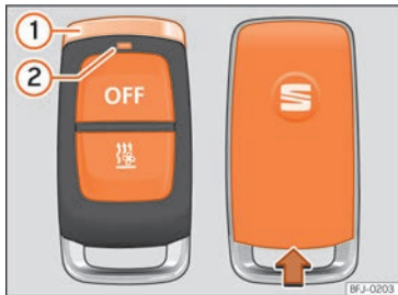
Fig. 138 Auxiliary heating: radio-operated remote control.
