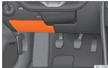
Fig. 49 Left hand drive vehicles: fuse box cover under the driver's side dashboard
