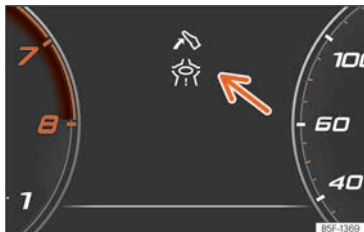
Fig. 58 Eco-efficient driving assistance indication (schematic representation).
