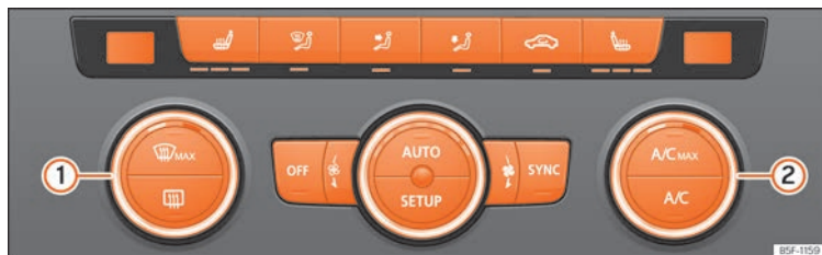
Fig. 134 In the centre console: Climatronic controls.
