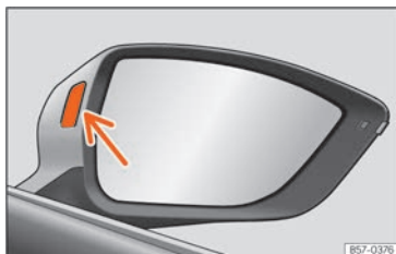
Fig. 178 Control lamp of the lane departure warning.
