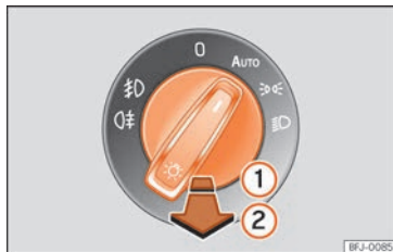
Fig. 97 Dash panel: lights control.
