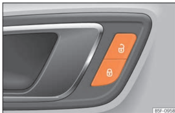
Fig.79 Driver's door: central locking switch.
