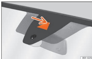
Fig. 159 On the windscreen: field of vision of the Lane Assist system.
