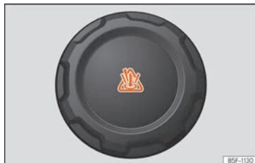
Fig. 215 Engine compartment: coolant expansion tank cap.
