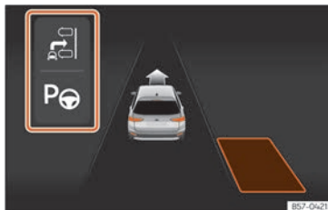
Fig. 185 On the instrument panel display: view of the parking assist system with reduced view.
