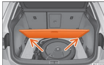
Fig. 120 Variable luggage compartment floor: inclined position.
