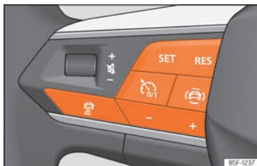
Fig. 168 On the multifunction steering wheel: buttons to operate the ACC
