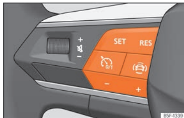
Fig. 164 On the multifunction steering wheel: buttons to operate the speed limiter.
