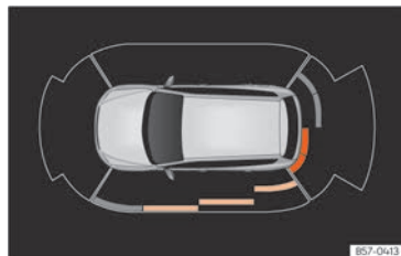
Fig. 192 Parking aid view on the Infotainment system display.
