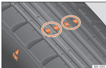
Fig. 220 Tyre profile: tread wear indicators.
