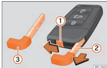
Fig. 75 Vehicle key: remove the emergency key.
