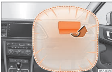
Fig. 15 Front passenger airbag located in dash panel.
