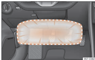
Fig. 19 On the driver side: airbag action radius for the knees.
