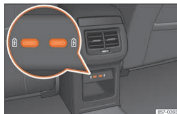
Fig. 148 Rear part of the centre console: USB connectors with power outlet function.
