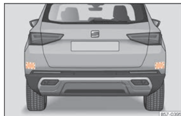
Fig. 161 Rear view of the vehicle: radar sensor zones.
