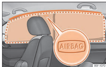
Fig. 22 Location of head-protection airbags.
