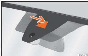
Fig. 160 On the windscreen: field of vision of the Lane Assist system.
