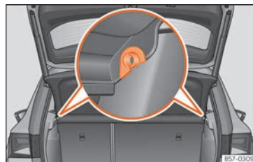
Fig. 117 In the luggage compartment: removing and fitting the shelf.
