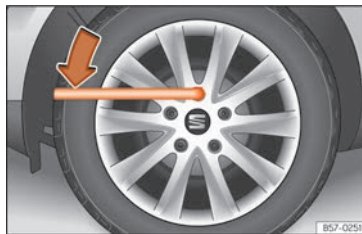
Fig. 219 Tyre change: slacken the wheel bolts.
