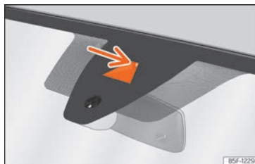
Fig. 109 On the windscreen: field of vision of the Lane Assist system camera.
