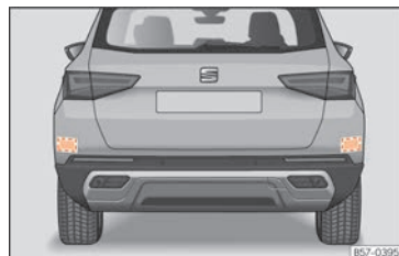
Fig. 110 Rear view of the vehicle: radar sensor areas.
