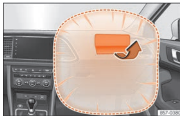
Fig. 28 Front passenger airbag located in dash panel.
