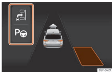
Fig. 138 On the instrument panel display: display of the assisted parking system with decreased visibility.
