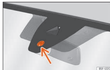
Fig. 88 Rain sensor sensitive surface
