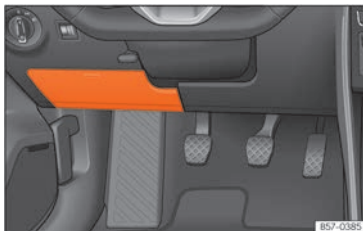
Fig. 196 On the dashboard on the driver side: lid of the fuse box.
