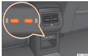
Fig. 156 Rear centre console: USB connectors with power socket function.
