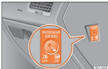
Fig. 29 Switch for activating and deactivating the front passenger airbag.
