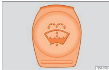
Fig. 205 In the engine compartment: blue cap of the windscreen washer tank.
