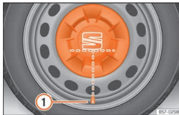
Fig. 216 Correct positioning of the central wheel trim for steel rims.
