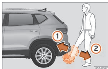
Fig. 62 Rear lid with sensor-controlled opening (Easy Open).
