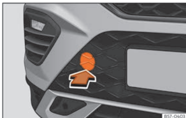
Fig. 192 Front bumper on right: remove the lid.
