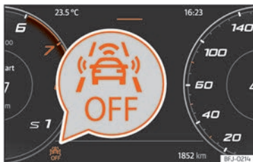
Fig. 122 On the screen of the instrument panel Front Assist switched off message.
