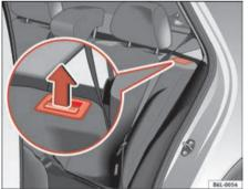
Fig. 75 Button for unlocking the rear backrest
