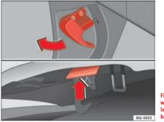
Fig. 122 Detail of footwell area on driver's side: lever for unlocking the bonnet.
