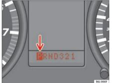
Fig. 100 Instrument panel display: Move the selector lever to position P. The selector lever lock is released as follows:
