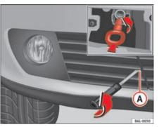
Fig. 160 Towing eye at the front of the vehicle
