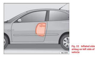
In some **side collisions** the side airbag is triggered on the impact side of the vehicle  $\Rightarrow$  fig. 22.
