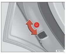
Fig. 44 Child safety lock on the left hand side door
