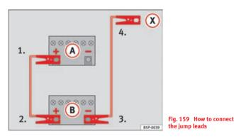
In  $\Rightarrow$  fig. 159, the flat battery is (A) and the charged battery (B).
