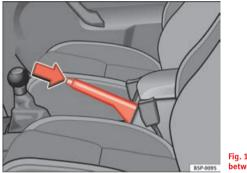
Fig. 101 Handbrake between the front seats
