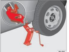
Fig. 136 Fitting the jack
