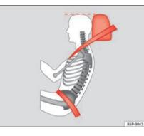
Fig. 14 Correct belt web and head restraint positions, viewed from side
