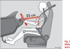
Fig. 1 The proper distance between driver and steering wheel
