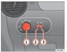
Fig. 56 Detail of instrument panel: lights, fog light and rear fog light switch
