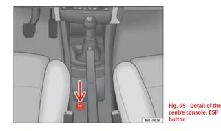
The Electronic Stabilisation Program (ESP) contains the electronic differential lock (EDL) and the traction control system (TCS). The ESP function works in conjunction with the ABS. Both warning lamps will light up if the ESP or ABS systems are faulty.
