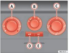
Fig. 91 On the instrument panel: air conditioner controls
