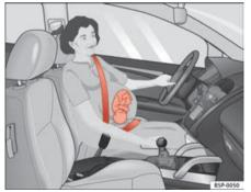
Fig. 15 Positioning seat belts during pregnancy
