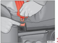
Fig. 16 Removing latch plate from buckle
