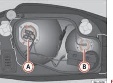
Fig. 145 Main beam lamp
