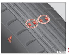
Fig. 130 Tyre tread wear indicators
