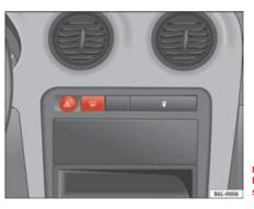
Fig. 58 Instrument panel: heated rear window switch The rear window heating only works when the engine is running. When it is switched on, a lamp lights up on the switch.
