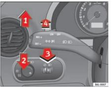
Fig. 60 Turn signal and main beam headlight lever
