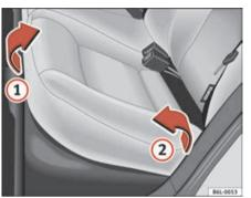
Fig. 74 Folding up the rear seat cushion
