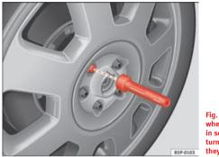
Fig. 137 Changing the wheel: hexagonal socket in screwdriver handle to turn the wheel bolts after they have been loosened
