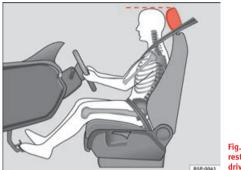
Fig. 2 Proper head restraint position for driver
