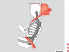
Fig. 70 Side view: head restraints and seat belts correctly adjusted
