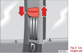
Fig. 6 Location of the belt height adjuster
