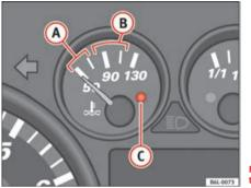
Fig. 33 Engine coolant temperature
