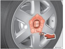
Fig. 132 Changing the wheel: Removing a hub cap
