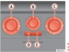
Fig. 90 On the instrument panel: air conditioner controls
