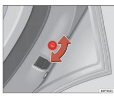
Fig. 45 Child safety lock on the right hand side door
