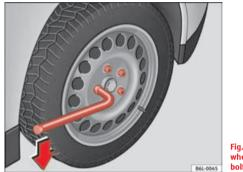
Fig. 134 Changing the wheel: loosen the wheel bolts
