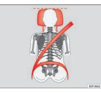
Fig. 13 Correct belt web and head restraint positions, viewed from front
