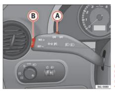
Fig. 103 Turn signal and main beam headlight lever switch and rocker switch for the cruise control
