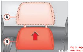
Fig. 5 Adjusting central rear head restraint
