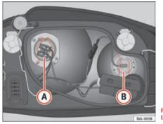
Fig. 144 Dipped headlight lamp
