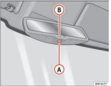
Fig. 67 Automatic antidazzle interior mirror.
