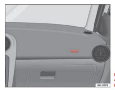
Fig. 18 Front passenger airbag located in dash panel The front airbag for the driver is located in the steering wheel  $\Rightarrow$  fig. 17 and the airbag for the front passenger is located in the dash panel  $\Rightarrow$  fig. 18. Airbags are identified by the text "AIRBAG".
