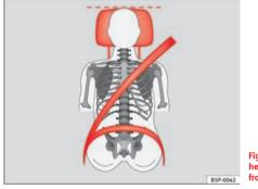
Fig. 3 Properly adjusted head restraint viewed from the front Adjust the head restraint properly to achieve maximum protection.
