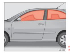
Fig. 24 Deployed curtain airbags
