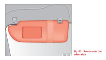
The sun visors for the driver and the front passenger can be pulled out of their mountings in the centre of the vehicle and turned towards the doors  $\Rightarrow$  fig. 63.
