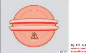
Fig. 126 In the engine compartment: Coolant expansion tank cap
