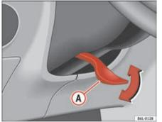
Fig. 93 Adjusting the steering wheel position
