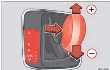
Fig. 171 Changing gear with Tiptronic.
