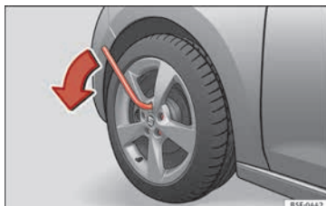
Fig. 65 Wheel: loosen the wheel bolts.
