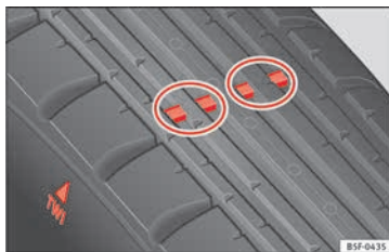
Fig. 189 Tyre tread wear indicators.
