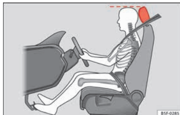
Fig. 76 Correct head restraint position for the driver.
