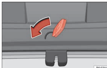
Fig. 5 IBIZA ST: Unlocking the rear lid manually.
