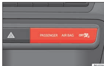
Fig. 86 Centre side of dash panel: control lamp for deactivated front passenger airbag in centre console
