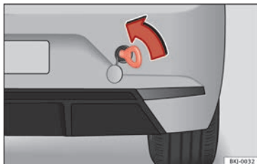
Fig. 93 Right side of the rear bumper: towline anchorage screwed in.
