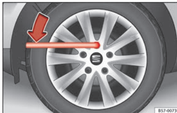
Fig. 66 Changing a wheel: loosen the wheel bolts.
