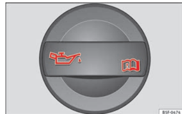
Fig. 54 In the engine compartment: Engine oil filler cap.
