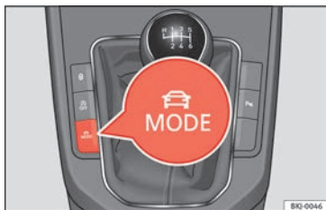
Fig. 170 Next to the gear lever. MODE button.
