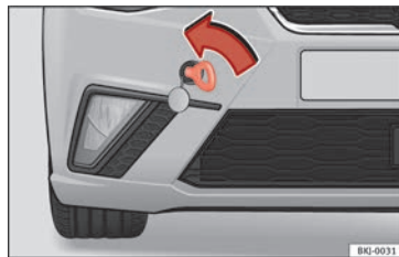
Fig. 91 Right side of the front bumper: tow-line anchorage screwed in.
