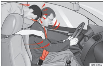
Fig. 85 The unbelted passenger in the rear seat is thrown forward violently, hitting the driver who is wearing a seat belt.
