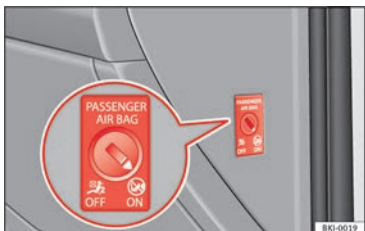
Fig. 19 Front passenger front airbag switch.
