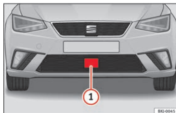
Fig. 164 On the front bumper: radar sensor.
