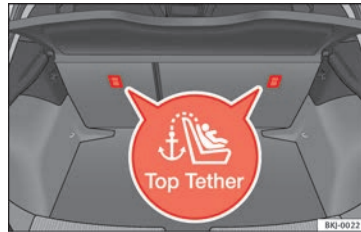
Fig. 27 Position of the Top Tether rings on the back of the rear seat.
