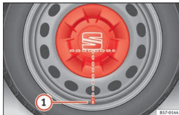
Fig. 63 Correct position of the central wheel trim for steel wheels.
