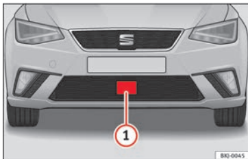
Fig. 158 On the front bumper: radar sensor.
