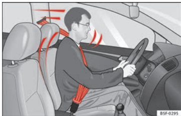
Fig. 83 Drivers with properly worn seat belts will not be thrown forward in the event of sudden braking.
