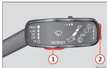
Fig. 39 Windscreen wiper lever: control buttons.
