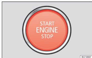
Fig. 149 In the lower part of the centre console: starter button.
