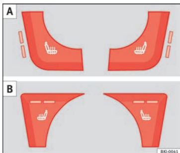
Fig. 130 In the centre console: front seats heating switch A ): version with Climatronic. B ): version with manual air conditioning.
