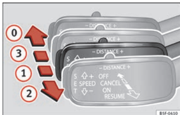
Fig. 165 On the left of the steering column: third lever for operating the Adaptive Cruise Control.
