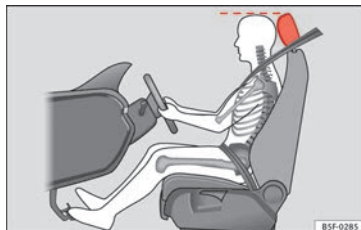
Fig. 78 Correct head restraint position for the driver.
