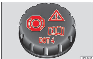
Fig. 56 Engine compartment: brake fluid reservoir cap.
