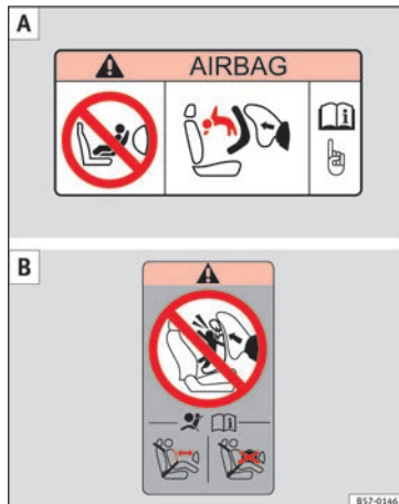
Fig. 24 Airbag stickers - version 2: on the front passenger's sun visor A and on the rear frame of the front passenger's door B .
