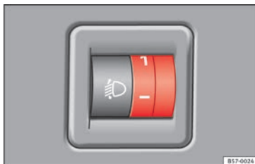
Fig. 125 Dash panel: headlight range control.
