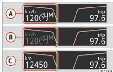
Fig. 154 On the instrument panel display: messages on the status of the speed limiter.
