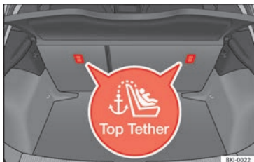
Fig. 29 Position of the Top Tether rings on the back of the rear seat.
