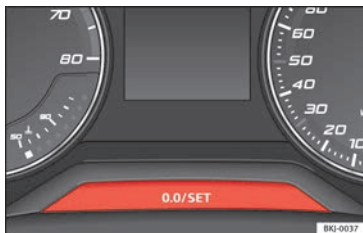
Fig. 107 Instrument panel: odometer and re-set button.
