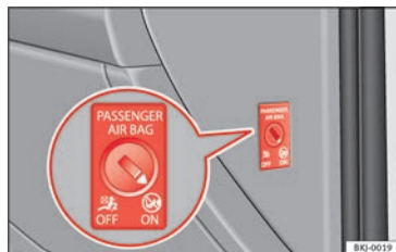
Fig. 88 Switch for activating and deactivating the front passenger airbag.
