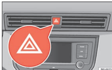
Fig. 34 Dash panel: switch for hazard warning lights.
