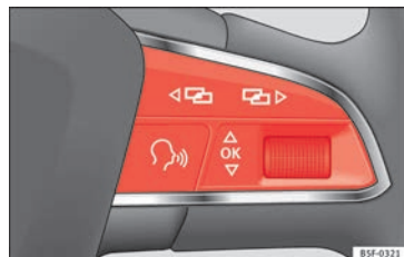
Fig. 40 Right side of multifunction steering wheel: control buttons.
