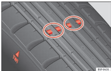
Fig. 195 Tyre tread wear indicators.
