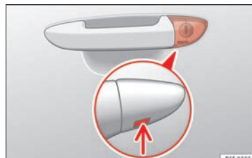
Fig. 3 Driver door lever: hidden lock cylinder.
