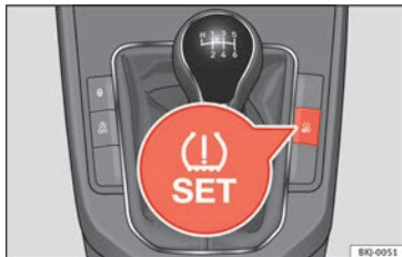
Fig. 197 Centre console: tyre monitoring system button.
