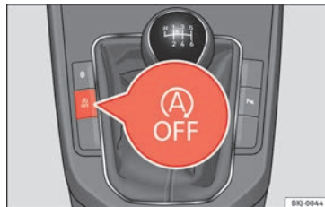
Fig. 152 Centre console: Start-Stop system button.
