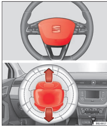
Fig. 17 Driver airbag located in steering wheel.
