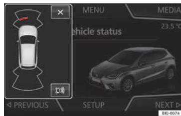
Fig. 174 Miniature indication of automatic activation.
