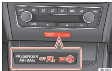
Fig. 89 Centre side of dash panel: control lamp for deactivated front passenger airbag in centre console.
