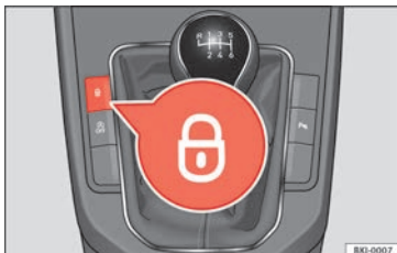
Fig. 2 Centre console: Central lock buttons.
