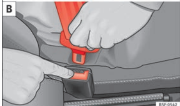
Fig. 13 Positioning and removing the seat belt buckle.
