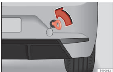
Fig. 71 Right side of the rear bumper: Towing ring.
