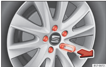
Fig. 65 Wheel: wheel bolts with caps.
