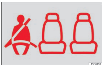
Fig. 82 Instrument panel: right rear seat occupied and corresponding seat belt fastened display.
