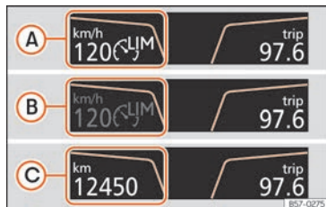
Fig. 228 On the instrument panel display: indications of the speed limiter status.
