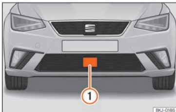
Fig. 232 On the front bumper: radar sensor.
