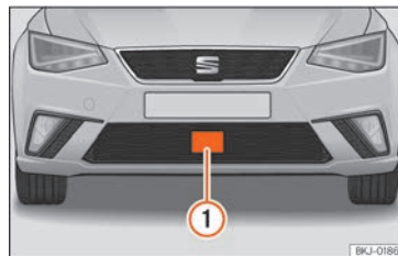
Fig. 237 On the front bumper: radar sensor.
