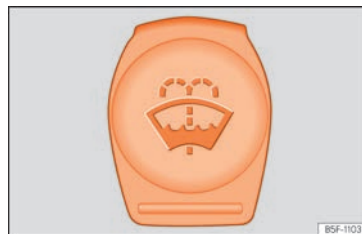
Fig. 63 In the engine compartment: cap of the windscreen washer tank.
