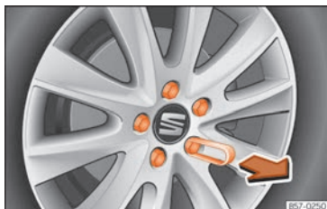
Fig. 73 Wheel: wheel bolts with caps.
