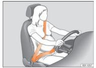
Fig. 13 Position of seat belt during pregnancu.
