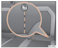
Fig. 26 Rear seat: slots die cut to access the ISOFIX / iSize securing rings.
