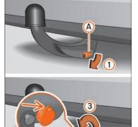
Fig. 257 Removing the tow hook
