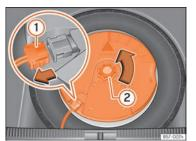
Fig. 280 In the luggage compartment: remove the subwoofer
