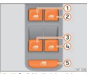
**Fig. 101** Detail of the driver's door: window controls.
