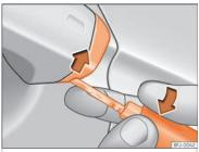
Fig. 96 Driver door handle: lever the cover off
