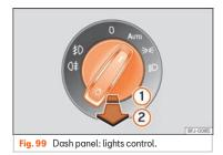
The warning lamps ≵0 or ()‡ also show, on the light switch or instrument panel, when the front fog lights are on.
