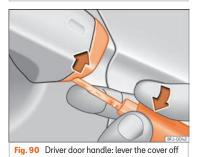
If the central locking system should fail to operate, the driver door can still be locked and unlocked by turning the key in the lock. As a general rule, when the driver door is locked manually all other doors are locked. When it is unlocked manually, only the driver door opens. Please observe the instructions relating to the anti-theft alarm system **»** page 105.
