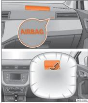
Fig. 15 Front passenger airbag located in dash panel.
