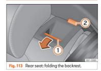
On split rear seats\*, the backrest can be lowered in two sections.
