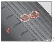
Fig. 152 Tyre tread wear indicators
