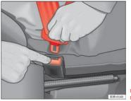
Fig. 15 Removing latch plate from buckle
