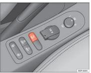
Fig. 130 Centre console: Switch for parking aid
