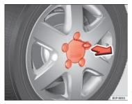
Fig. 155 Changing the wheel: Removing a hub cap
