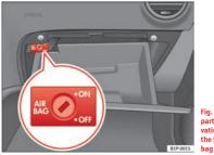
Fig. 25 In the glove compartment: switch for activating and deactivating the front passenger air-
