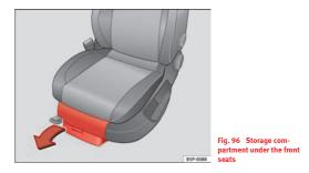
The locker\*  $\Rightarrow$  fig. 96 (A) is opened by pulling on the cover.
