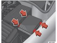
Fig. 161 Fuse box cover in engine compartment
