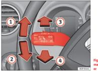
Fig. 76 Turn signal and main beam headlight lev-
