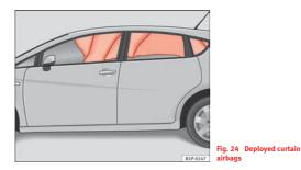
During some **side collisions** the curtain airbag is triggered on the impact side of the vehicle  $\Rightarrow$  fig. 24.
