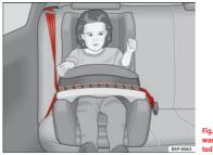
Fig. 28 A category 1 forward-facing child seat fitted on the rear seat.
