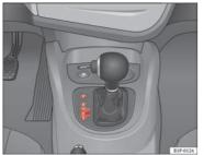
Fig. 123 Centre console: Selector lever for automatic gearbox / DSG automatic gearbox
