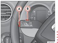
Fig. 132 Turn signal and main beam headlight lever: switch and rocker switch for the cruise control
