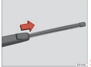
Fig. 149 Removing rear window wiper blade
