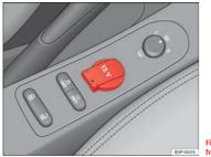
Fig. 100 Power socket, front centre console
