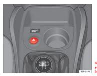
Fig. 75 Dash panel: switch for hazard warning lights
