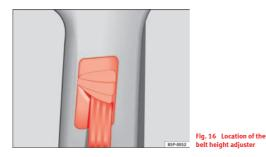
The seat belt adjuster for the front seats can be used to adjust the proper belt position at the shoulder.
