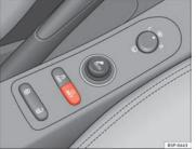
Fig. 50 Centre console: tyre monitor system button
