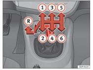
Fig. 122 Detailed view of the centre console: gear shift pattern of a 6-speed manual gearbox
