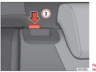
Fig. 94 Folding up the rear backrest
