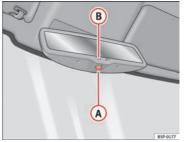
Fig. 85 Automatic antidazzle interior mirror.
