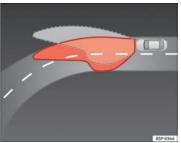
Fig. 74 Cornering lighting using adaptive headlights
