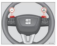
Fig. 128 Steering wheel with levers for automatic gearbox
