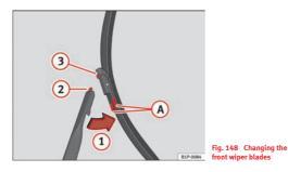
Changing wiper blades can be done in both the rest and horizontal positions. Ensure that the wiper blades are not frozen.
