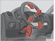
Fig. 114 Adjusting the steering wheel position
