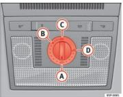
Fig. 69 Roof lining description: sliding/tilting sunroof rotary knob
