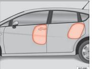
Fig. 22 Illustration of principle: inflated side airbags on left side of vehicle
