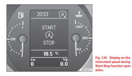
When the engine is turned off by the Start-Stop function, this is displayed on the instrument panel.
