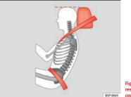
Fig. 88 Side view: head restraints and seat belts correctly adjusted
