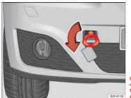
Fig. 182 The front right section of the vehicle: Fitting the front towing eve
