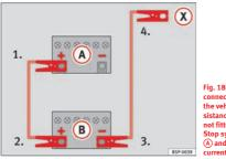
Fig. 180 Diagram for connecting jump leads if the vehicle providing assistance the current is not fitted with the Start-Stop system: flat battery (**A**) and battery providing current (**B**).
