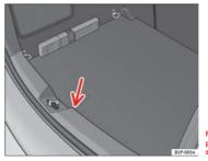
Fig. 154 Luggage compartment. Access to the spare wheel
