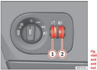
Fig. 73 Dash panel: regulation for instrument and switch illumination and headlight range control
