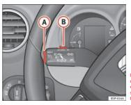
Fig. 135 Turn signal and main beam headlight lever: switch and rocker switch for the cruise control
