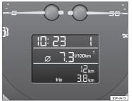
Fig. 40 Digital instrument panel display The multifunction system uses two automatic memories: **1** - **Actual memory** and **2** - **Total memory**. The selected memory will be shown in the upper right-hand corner of the display.
