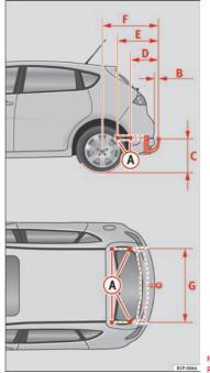
Fig. 137 Attachment points for towing bracket
