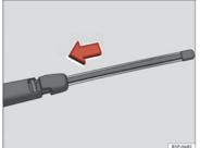
Fig. 150 Fitting the rear window wiper blade
