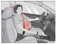
Fig. 14 Positioning seat belts during pregnancy
