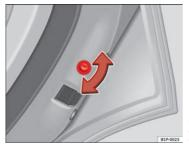
Fig. 60 Childproof lock on the right hand side door This function is independent of the vehicle electronic opening and locking systems. It only affects rear doors. It can only be activated and deactivated manually, as described below:
