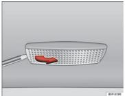
Fig. 178 Removing sun visor light
