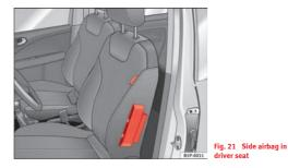
The side airbags are located in the backrest cushions of the driver seat  $\Rightarrow$  fig. 21 and the front passenger seat as well as in the rear seats. The locations are identified by the text "AIRBAG" in the upper region of the backrests.
