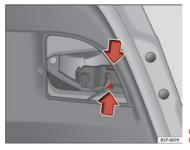
Fig. 172 Removing the bulb holder
