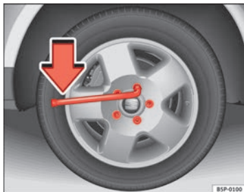
Fig. 156 Changing the wheel: loosen the wheel bolts
