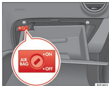
Fig. 25 In the glove compartment: switch for activating and deactivating the front passenger airbag
