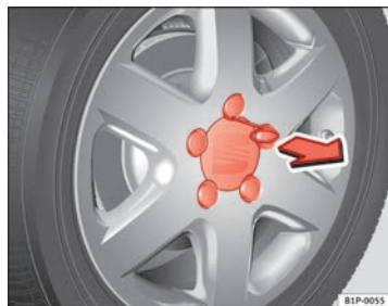
Fig. 155 Changing the wheel: Removing a hub cap
