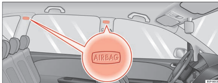
Fig. 23 Location of head airbags on the left side of the vehicle
