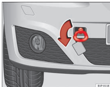
Fig. 182 The front right section of the vehicle: Fitting the front towing eye
