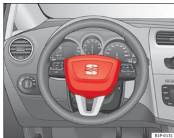
Fig. 17 Driver airbag located in steering wheel
