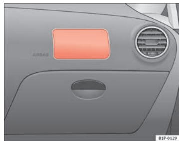
Fig. 18 Front passenger airbag located in dash panel
