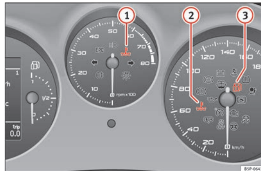
Fig. 49 Instrument panel indicator and warning lamps in vehicles with LPG.
