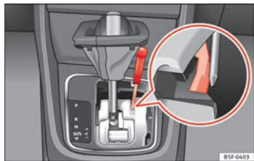
Fig. 127 Selector lever: manual release from position P.
