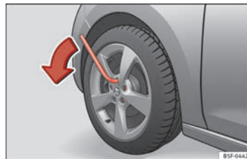
Fig. 172 Wheel: loosen the wheel bolts.
