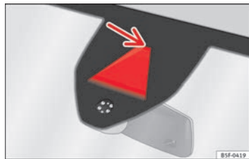
Fig. 147 In the wind-screen: field of vision of the Lane Assist system camera.
