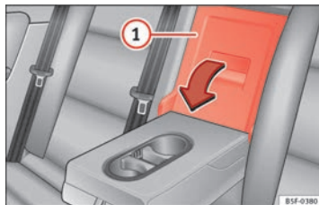
Fig. 104 On the rear seat backrest: opening the tailboard.
