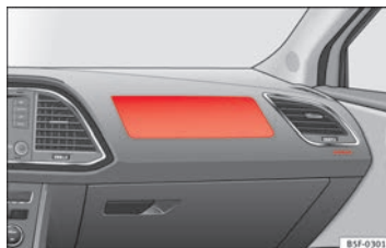
Fig. 20 Front passenger airbag located in dash panel.
