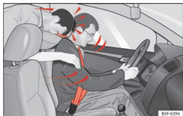
Fig. 10 The unbelted passenger in the rear seat is thrown forward violently, hitting the driver wearing a seat belt.
