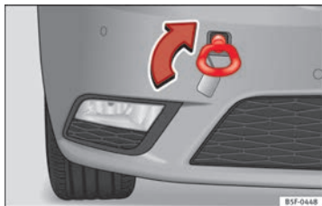
Fig. 178 Right side of the front bumper: towline anchorage screwed in.
