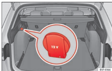
Fig. 90 Detailed view of the side trim in the luggage compartment: 12-volt power socket (applies only to the LEON ST model).
