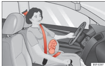
Fig. 15 Positioning seat belts during pregnancy.
