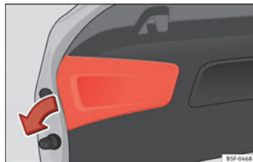
Fig. 199 Remove the cover from the rear lid.
