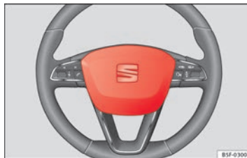
Fig. 19 Driver airbag located in steering wheel.
