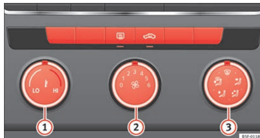
Fig. 118 In the centre console: heating system and fresh air controls.
