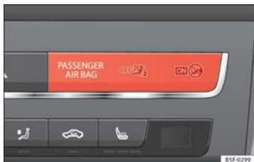
Fig. 24 Warning lamp for disabling the front passenger airbag.
