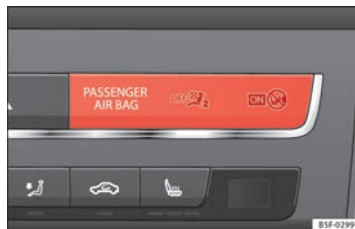
Fig. 16 Control lamp for disabling the front passenger front airbag on the dash panel
