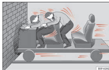
Fig. 8 The vehicle hits the wall: the vehicle occupants are not wearing seat belts
