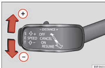
Fig. 196 On the left of the steering column: third lever for operating the Adaptive Cruise Control.
