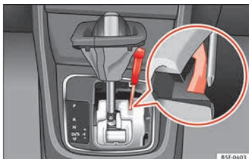
Fig. 55 Selector lever: manual release from position P.
