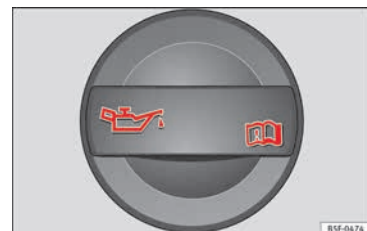
Fig. 61 In the engine compartment: Engine oil filler cap
