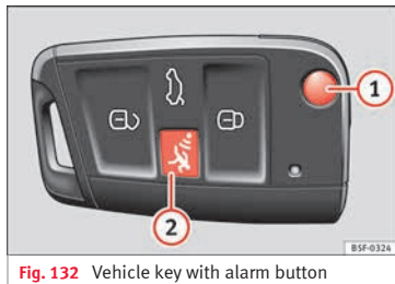
Fig. 132 Vehicle key with alarm button
