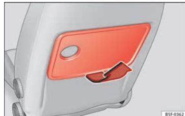
Fig. 154 Left-hand front seat: folding table.
