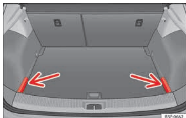
Fig. 162 In the luggage compartment: covers for storing the rear shelf.
