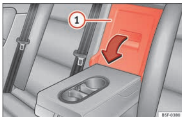
Fig. 170 On the rear seat backrest: opening the tailboard.
