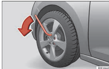
Fig. 73 Wheel: loosen the wheel bolts.
