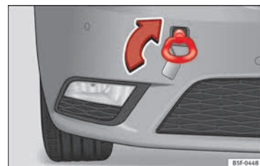
Fig. 76 Right side of the front bumper: towline anchorage screwed in.
