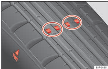
Fig. 238 Tyre tread: tread wear indicators
