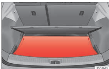
Fig. 163 In the luggage compartment: fitting the storage compartment shelf.
