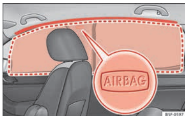
Fig. 28 Location of head-protection airbags.
