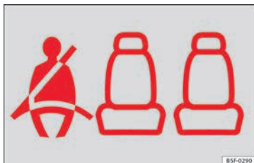
Fig. 88 Instrument panel: right rear seat occupied and corresponding seat belt fastened display.
