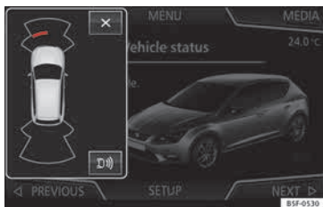
Fig. 215 Miniature indication of automatic activation
