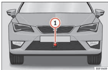
Fig. 195 On the front bumper: radar sensor.
