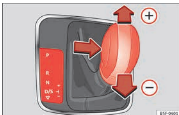
Fig. 188 Centre console: changing gear with tiptronic
