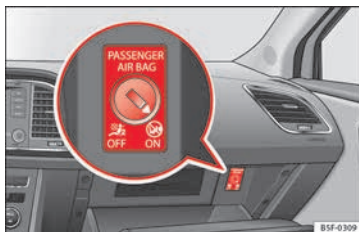
Fig. 95 Front passenger front airbag switch.
