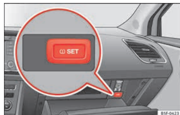
Fig. 241 Glove compartment: tyre control switch.
