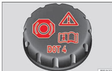
Fig. 63 Engine compartment: brake fluid reservoir cap
