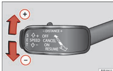
Fig. 197 On the left of the steering column: third lever for operating the Adaptive Cruise Control.
