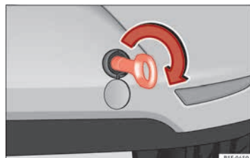
Fig. 100 Right side of the rear bumper: towline anchorage screwed in.
