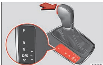
Fig. 54 Automatic gearbox: selector lever positions.
