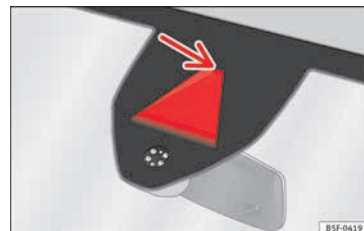
Fig. 208 In the windscreen: field of vision of the Lane Assist system camera.
