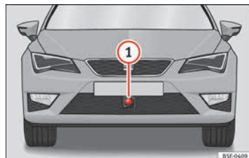
Fig. 203 On the front bumper: radar sensor.
