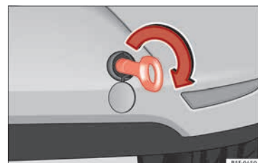
Fig. 77 Right side of the rear bumper: towline anchorage screwed in.
