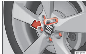
Fig. 71 Wheel: wheel bolts with caps.
