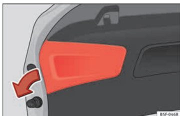
Fig. 118 Remove the cover from the boot lid.
