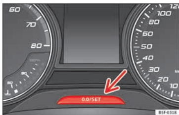
Fig. 125 Instrument panel: odometer and reset button.
