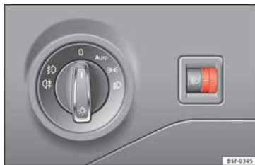
Fig. 140 Next to the steering wheel: Headlight range control
