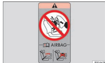
Fig. 30 On the rear frame of the passenger side door: airbag sticker.
