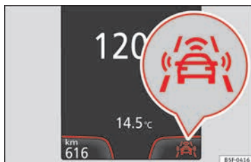
Fig. 204 On the instrument panel display: Front Assist switched off message.
