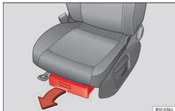
Fig. 153 Storage compartment under the front seats.
