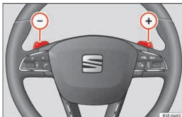
Fig. 189 Steering wheel: automatic gearbox levers
