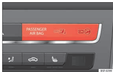
Fig. 94 Control lamp for disabling the front passenger front airbag on the dash panel
