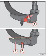
Fig. 223 Standby position: Position of the lever and the release bolt
