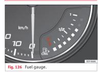
Displays (2) and (6) **\*\*\*** Fig. 124 only work when the ignition is switched on. When the display reaches the reserve mark, the lower diode lights up in red and the control lamp (2) appears **\*\*** page 104. When the fuel level is very low, the lower diode flashes in red. The yellow control lamp  $\boxplus$  lights up when the reserve level has been reached.
