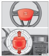
Fig. 21 Driver airbag located in steering wheel.
