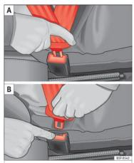
Fig. 92 Positioning and removing the seat belt buckle.
