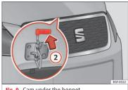
Fig. 9 Cam under the bonnet
