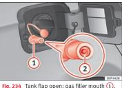
Fig. 234 Tank flap open: gas filler mouth (1) filler mouth retainer (2)
