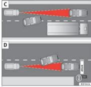
**Fig. 202** (C) Vehicle changing lanes. (D) One vehicle turning and another stationary.
