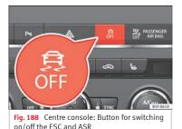
The ESC is switched on automatically when the engine is started, and only works when the engine is running and includes the ABS, EDS and ASR systems.
