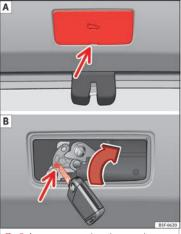
Fig. 7 Luggage compartment: access to manual release.
