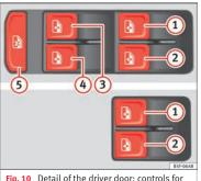
**Fig. 10** Detail of the driver door: controls fo the windows.
