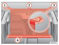
Fig. 170 In the luggage compartment: net partition hooked into the rear seat backrests.
