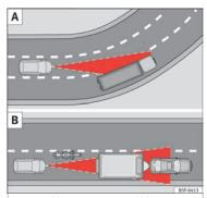
Fig. 201 (A) Vehicle on a bend. (B) Motorcyclist ahead out of range of the radar sensor.
