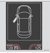
Fig. 51 On the instrument panel display: door open.
