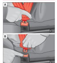
**Fig. 16** Positioning and removing the seat belt buckle.
