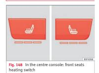
The seat cushions can be heated electrically when the ignition is switched on. The backrest is also heated in some versions.
