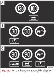
Fig. 212 On the instrument panel display: examples of speed limits or overtaking prohibitions with their respective additional signs.
