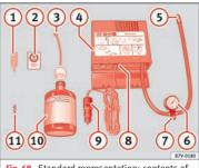
**Fig. 68** Standard representation: contents of the anti-puncture kit.
