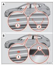
Fig. 183 Leon/Leon SC: attachment points for the roof railings for the roof carrier system.
