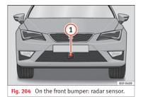
A radar sensor is installed on the front bumper to determine the traffic situation **>>> Fig. 204 (1)**. This sensor can detect vehicles in front up to a distance of approximately 120 m.
