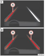
**Fig. 208** On the instrument panel display: Indication on the Lane Assist system display (example 2).
