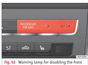
**Fig. 52** Warning lamp for disabling the front passenger airbag.
