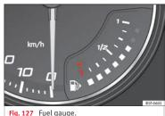
The display ( $\bigcirc$ ) **>>> Fig. 124** only works when the ignition is switched on. When the display reaches the reserve mark, the lower diode lights up in red and the control lamp  $\square$  appears **>>> page 104**. When the fuel level is very low, the lower diode flashes in red.
