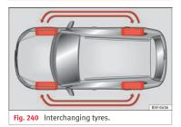
To ensure that the wear is equal on all tyres the wheels should be changed round from time to time according to the system **>>> Fig. 240.** The useful life of all the tyres will then be about the same time.
