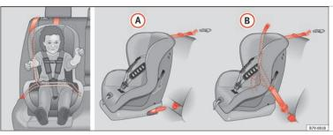
Fig. 31 On the rear seats: Possible installations for the child seat.
