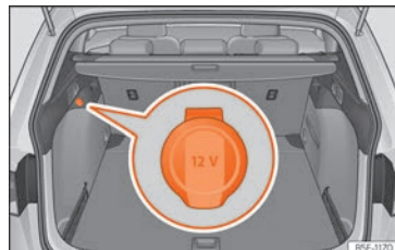
Fig. 168 Detail of the side lining of the luggage compartment: 12 volt power socket (valid only for the Leon Sportourer ST model).
