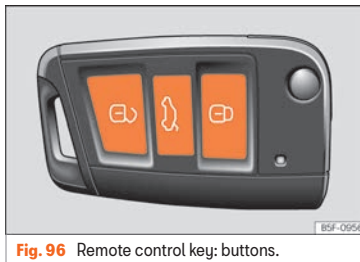
Fig. 96 Remote control key: buttons.
