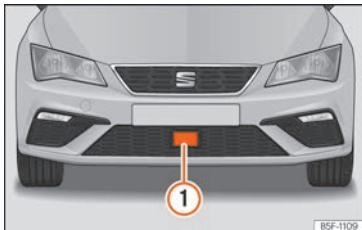
Fig. 275 On the front bumper: radar sensors.
