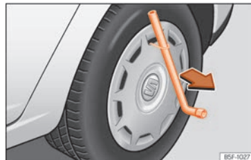
Fig. 35 Remove the wheel cover.
