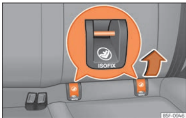
Fig. 28 Rear seat: ISOFIX securing rings.
