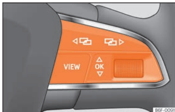
Fig. 85 Right side of the multifunction steering wheel: buttons to the menus and information displays on the instrument panel.
