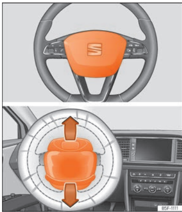
Fig. 15 Driver airbag located in steering wheel.
