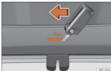
Fig. 106 Detail of the luggage compartment: emergency unlocking (LEON model).
