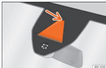
Fig. 281 On the windscreen: field of vision of the Lane Assist system.
