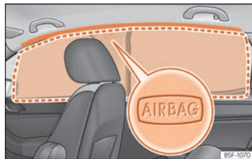
Fig. 23 Location of head-protection airbags.
