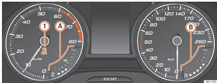
Fig. 81 Analogue instrument panel: natural gas gauge
