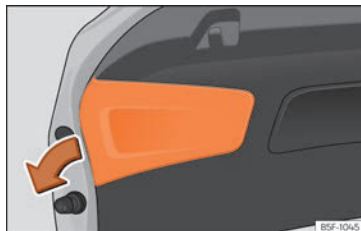
Fig. 67 Remove the cover from the rear lid
