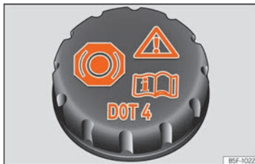
Fig. 321 Engine compartment: brake fluid reservoir cap.
