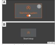
Fig. 163 On the Infotainment system screen.: Start-Stop system connected. A View in the main menu. B View with the Infotainment system off.
