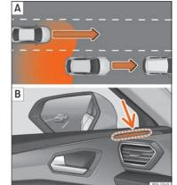
Fig. 190 Schematic representation: A Passing situation with traffic behind the vehicle. B Indication of the lane departure warning in the control lamp on the left side.
