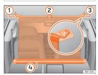
Fig. 141 In the luggage compartment: net partition hooked in place with the rear seat backs folded down.
