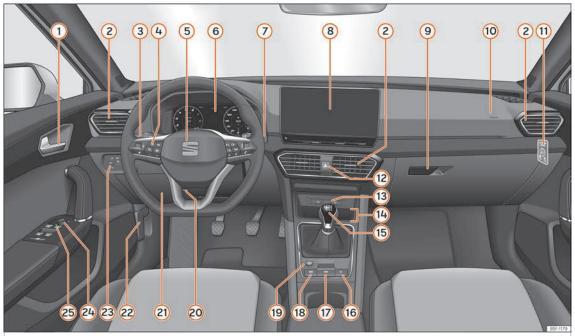
Fig. 58 Instruments and controls.
