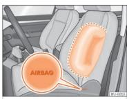
Fig. 26 Side airbag in driver's seat.
