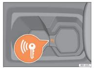
Fig. 162 In the centre console: emergency start
