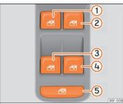
Fig. 98 Detail of the driver's door: window controls.
