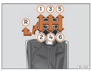
Fig. 164 Gear shift pattern of a 6-speed manual gearbox
