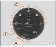
Fig. 65 Digital instrument panel: Power meter
