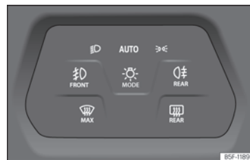
Fig. 101 Dash panel: lights control.
