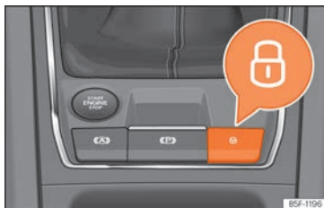
Fig. 86 In the centre console: central locking switch
