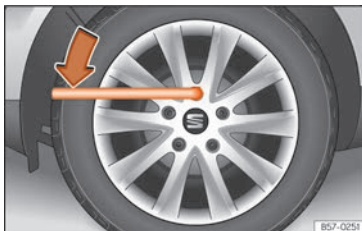
Fig. 43 Wheel change: loosen the wheel nuts.
