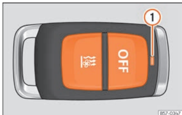
Fig. 151 Auxiliary heating: radio-operated remote control.
