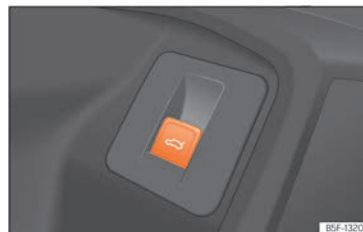
Fig. 94 On the driver's door: button to open and close the rear lid.
