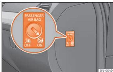
Fig. 20 Switch for activating and deactivating the front passenger airbag.
