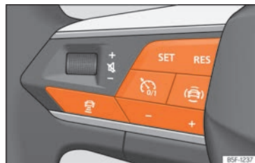
Fig. 179 On the multifunction steering wheel: buttons to operate the ACC
