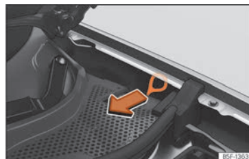
Fig. 213 Between the left wing panel and the engine bonnet hinge: Charging connector manual release mechanism puller.
