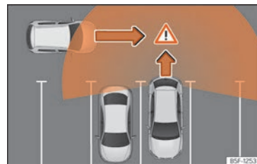
Fig. 192 Schematic representation of the rear cross traffic alert assistant: zone monitored around the vehicle while leaving a parking space.
