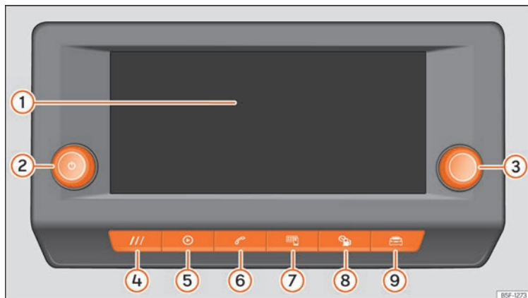
Fig.153 Overview: control unit and indication in the 8.25-inch version
