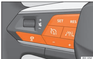
Fig. 187 Left side of the multifunction steering wheel: buttons for operating Travel Assist.
