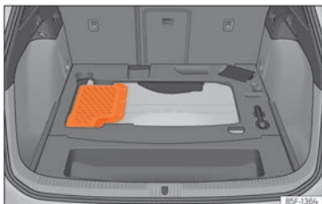
Fig. 231 Location of the battery in the luggage compartment
