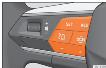
Fig. 173 On the multifunction steering wheel: buttons to operate the speed limiter.
