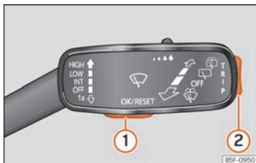
Fig. 71 Wiper lever: control keys.
