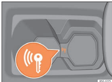
Fig. 162 In the centre console: emergency start.
