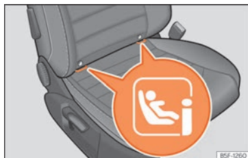
Fig. 33 Front passenger seat: ISOFIX/i-Size securing rings.
