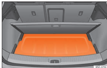
Fig. 124 In the luggage compartment: fitting the rear shelf.
