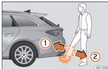
Fig. 95 Rear lid with sensor-controlled opening [Easy Open].
