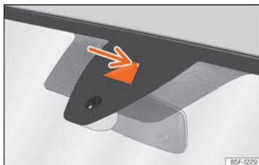
Fig. 169 On the windscreen: field of vision of the Lane Assist system.
