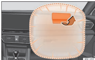
Fig. 19 Front passenger airbag located in dash panel.
