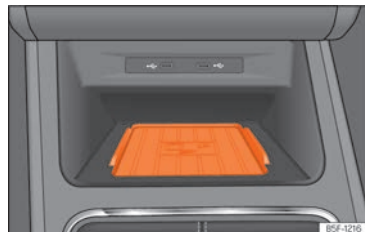
Fig. 158 In the centre console: pad for the mobile phone connection.
