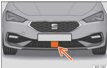
Fig. 167 On the front bumper: radar sensors.
