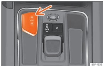
Fig. 81 Centre console: vehicle key socket.
