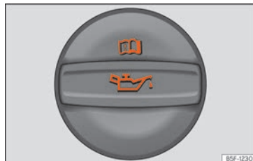
Fig. 225 In the engine compartment: Engine oil filler cap.
