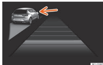
Fig. 181 On the instrument panel display: ACC active, vehicle detected in an outer lane.
