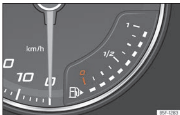
Fig. 67 Analogue instrument panel: fuel gauge
