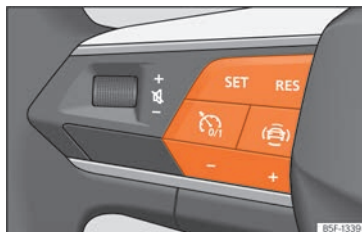
Fig. 174 On the multifunction steering wheel: buttons to operate the speed limiter.
