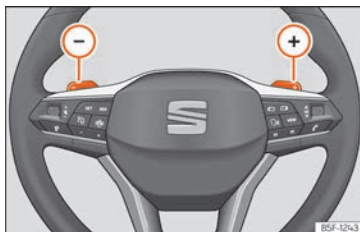
Fig. 166 Steering wheel: automatic transmission levers
