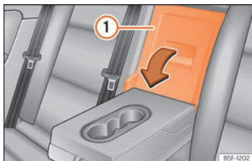
Fig. 136 In the rear seat backrest: opening the trapdoor.
