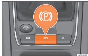
Fig. 195 In the lower part of the centre console: electronic parking brake button
