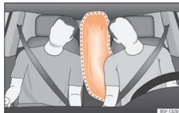
Fig. 25 Fully inflated central airbag (deployment zone).
