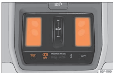
Fig. 104 Detail of roof lining: front lighting of the passenger compartment.
