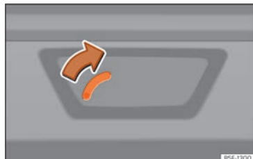
Fig. 97 Detail of the luggage compartment: manual release mechanism (Leon Sportstourer).
