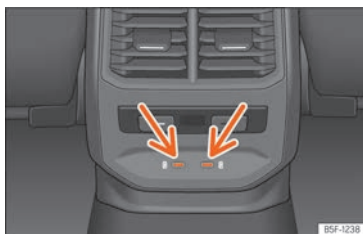
Fig. 160 Rear part of the centre console: USB connectors with power outlet function.
