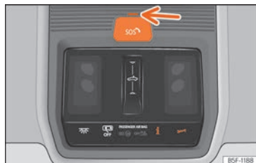
Fig. 37 On the roof console: voice service controls
