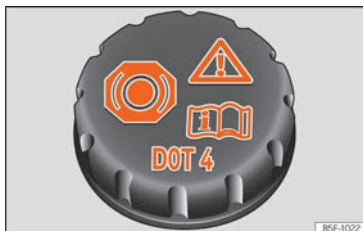
Fig. 229 Engine compartment: brake fluid reservoir cap.
