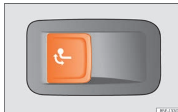
Fig. 206 On the left side of the luggage compartment: button for unlocking the tow hook.
