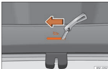
Fig. 96 Detail of the luggage compartment: emergency release (Leon).
