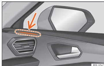
Fig. 189 Control lamp of the lane departure warning.
