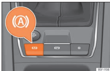
Fig. 196 In the lower part of the centre console: Auto Hold function button.
