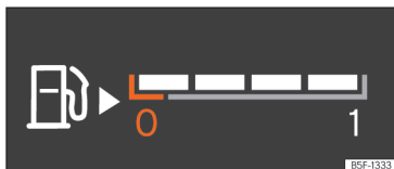
Fig. 68 Digital instrument panel: fuel level indicator located in different positions depending on the view.
