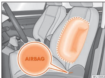
Fig. 26 Side airbag in driver's seat.
