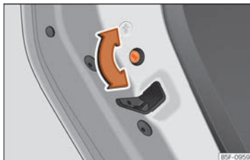
Fig. 91 Childproof lock on the left hand side door.
