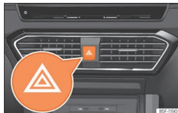
Fig. 103 Dash panel: hazard warning lights switch
