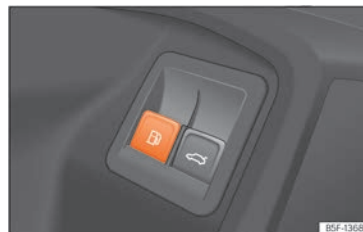
Fig. 217 Driver's door: tank flap release.
