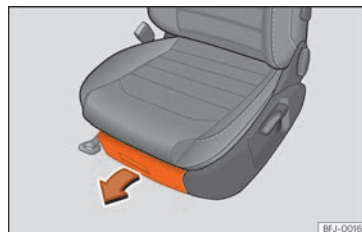
Fig. 145 Drawer under the front seat
