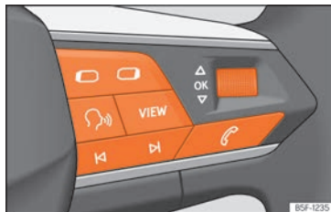
Fig. 70 Right side of the multifunction steering wheel: buttons to the menus and information displays on the instrument panel.
