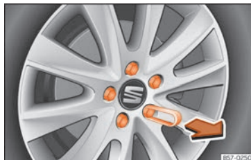
Fig. 41 Wheel: wheel nuts with caps.
