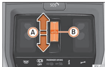
Fig. 99 On the interior roof lining: sunroof button.
