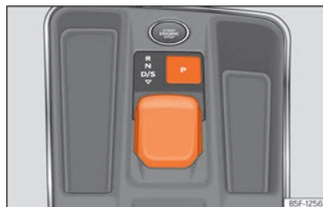
Fig. 167 In the centre console: selector lever.
