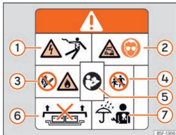
Fig. 210 High-voltage battery warning lettering.
