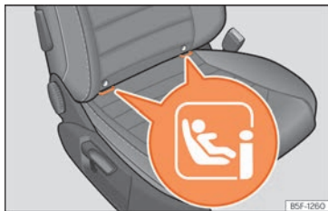
Fig. 33 Front passenger seat: ISOFIX/i-Size securing rings.
