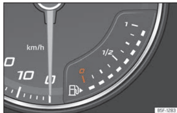
Fig. 67 Analogue instrument panel: fuel gauge
