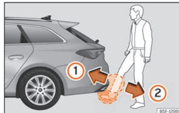
Fig. 96 Rear lid with sensor-controlled opening (Easy Open).
