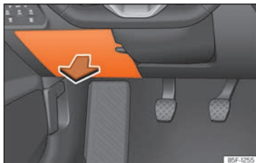
Fig. 55 On the driver's side dashboard: fuse box cover.
