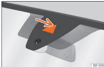
Fig. 171 On the windscreen: field of vision of the Lane Assist system.
