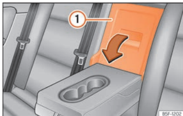
Fig. 137 In the rear seat backrest: opening the trapdoor.
