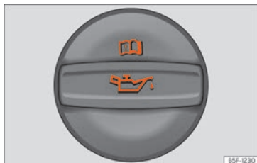
Fig. 231 In the engine compartment: Engine oil filler cap.
