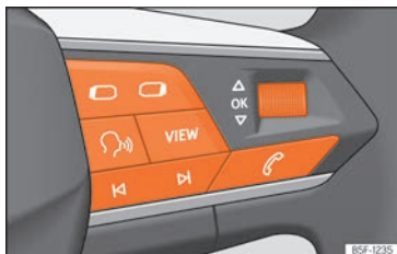
Fig. 71 Right side of the multifunction steering wheel: buttons to the menus and information displays on the instrument panel.
