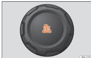
Fig. 234 Engine compartment: coolant expansion tank cap.
