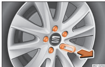
Fig. 41 Wheel: wheel nuts with caps.
