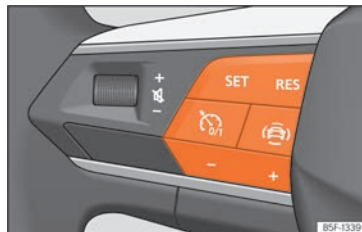
Fig. 176 On the multifunction steering wheel: buttons to operate the speed limiter.
