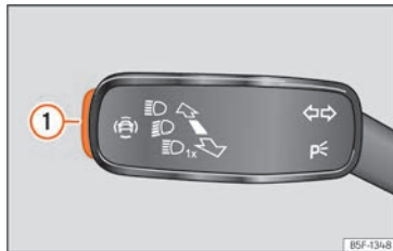
Fig. 72 On the turn signal and main beam lever: button for driver assistance systems [depending on versions].
