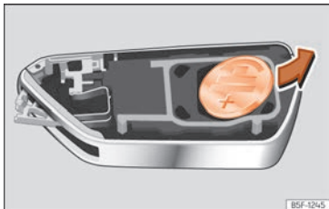
Fig. 85 Vehicle key: removing the battery.
