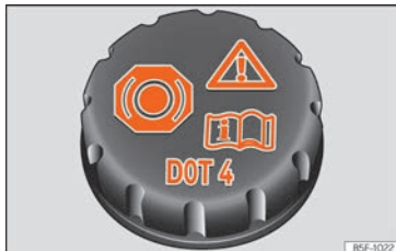
Fig. 235 Engine compartment: brake fluid reservoir cap.
