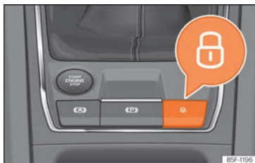
Fig. 87 In the centre console: central locking switch
