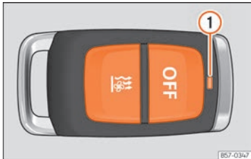
Fig. 153 Auxiliary heating: radio-operated remote control.
