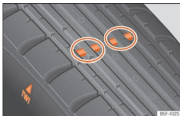
Fig. 241 Tyre profile: tread wear indicators.
