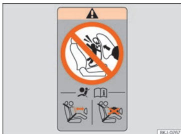
Fig. 31 Airbag sticker: on the rear frame of the passenger side door
