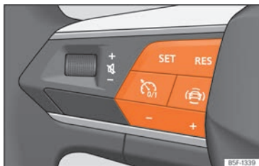
Fig. 175 On the multifunction steering wheel: buttons to operate the speed limiter.
