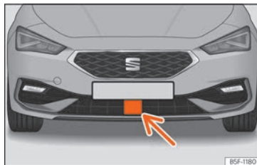
Fig. 169 On the front bumper: radar sensors.
