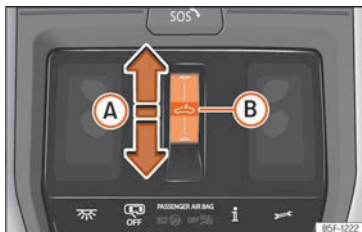
Fig. 100 On the interior roof lining: sunroof button.
