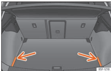
Fig. 124 In the luggage compartment: covers for storing the rear shelf.
