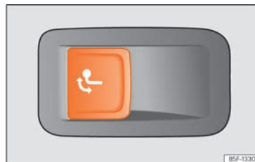
Fig. 207 On the left side of the luggage compartment: button for unlocking the tow hook.
