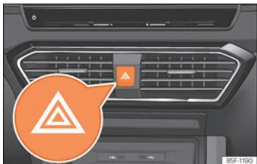
Fig. 104 Dash panel: hazard warning lights switch
