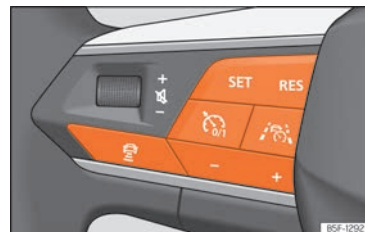
Fig. 188 Left side of the multifunction steering wheel: buttons for operating Travel Assist.
