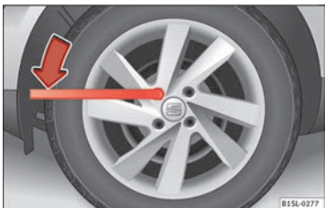
Fig. 52 Changing a wheel: Slacken the wheel bolts.
