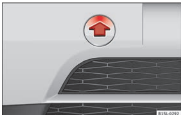
Fig. 79 On the right-hand side of the front bumper: Remove the cover.
