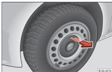
Fig. 49 Remove the hubcap of the steel wheel trim
