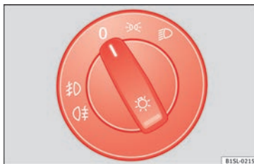
Fig. 107 Next to the steering wheel: diagram of some of the types of light switch
