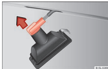
Fig. 89 Number plate light: Remove the bulb holder.
