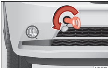
Fig. 80 On the right-hand side of the front bumper: Screw in the towline anchorage.
