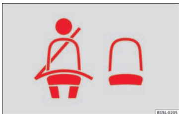
Fig. 66 Indication of seat belt status in the rear seats on the instrument panel display
