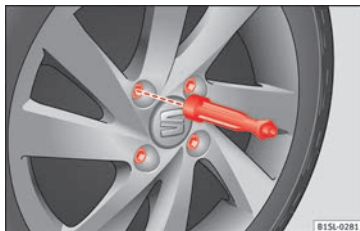
Fig. 56 Changing a wheel: loosen wheel bolts with the socket at the end of the wheel brace
