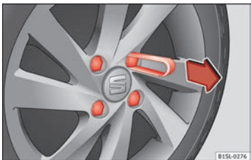
Fig. 51 Removing the wheel bolt caps
