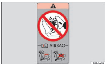
Fig. 24 On the rear frame of the passenger side door: airbag sticker.
