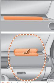
Fig. 20 Location and deployment area of the front airbag for the passenger.
