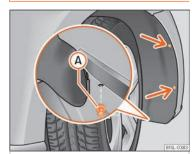
Fig. 87 In the front right arch trim: remove the retaining screws (arrows) and take out the expansive rivet (A).
