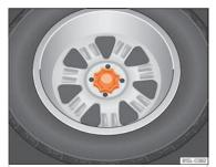
**Fig. 190** In the boot: hand controlled wheel for securing the spare wheel
