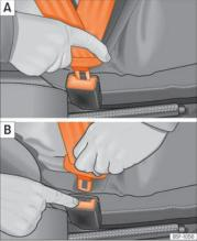
Fig. 73 Positioning and removing the seat belt buckle
