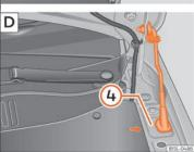
Fig. 10 C: Bonnet securing rod in the bonnet. D: Bonnet supported by the bonnet securing rod
