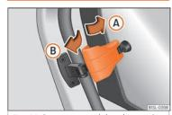
**Fig. 109** Lever to open and close the rear window
