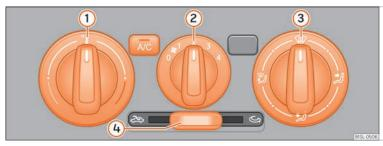
Fig. 39 Centre console, top section: controls for the manual air conditioning and the heating and fresh air system.
