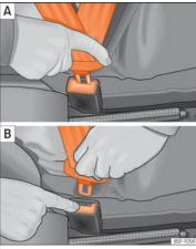
**Fig. 15** Positioning and removing the seat belt buckle.
