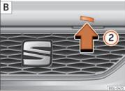
Fig. 9 A: Release lever in the footwell on the driver side B: Release lever on the bonnet
