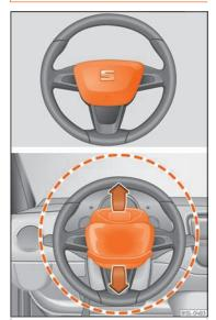
**Fig. 19** Location and deployment area of the front airbag for the driver.
