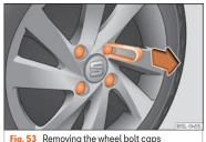
Fig. 53 Removing the wheel bolt caps
