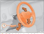
Fig. 18 Mechanical steering wheel adjustment
