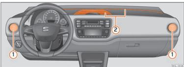
Fig. 141 On the dash panel air vents.
