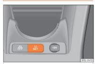
Fig. 189 Centre console: tyre monitoring system button.
