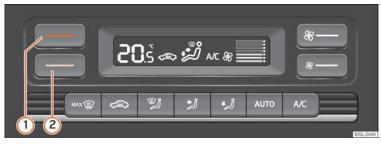
Fig. 142 In the centre console, top section: Climatronic control panel.
