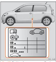
Fig. 187 Position of tyre pressure specification plate
