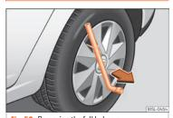
Fig. 52 Removing the full hubcap
