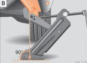
Fig. 57 Jack mounted on the left rear part of the vehicle
