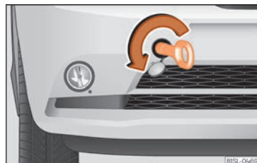
Fig. 43 Right side of the front bumper: towline anchorage screwed in.
