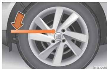
Fig. 33 Tyre change: slacken the wheel bolts.
