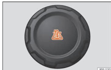
Fig. 162 Engine compartment: coolant expansion tank cap.
