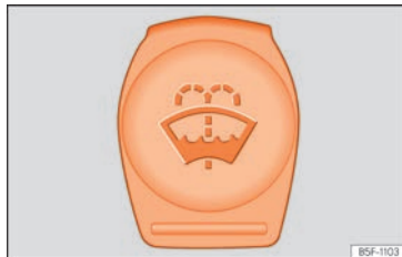
Fig. 164 In the engine compartment: cap of the windscreen washer tank.
