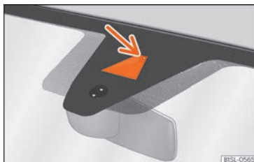
Fig. 141 On the windscreen: field of vision of the Lane Assist system camera.
