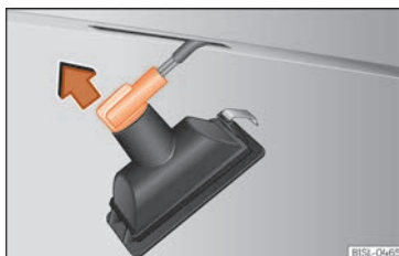
Fig. 55 Number plate light: detach the bulb holder.
