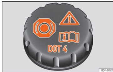
Fig. 163 Engine compartment: brake fluid reservoir cap.
