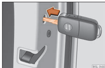
Fig. 71 Emergency locking of the vehicle using the vehicle key
